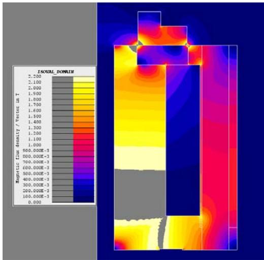
Figure 5. Simulation showing the saturation in the inside part of the actuator (half of the section is shown)
