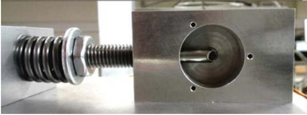
Figure 8. 450N radial loading of the pin
