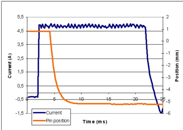
Figure 9. Record of command current and pin position during a typical actuation
