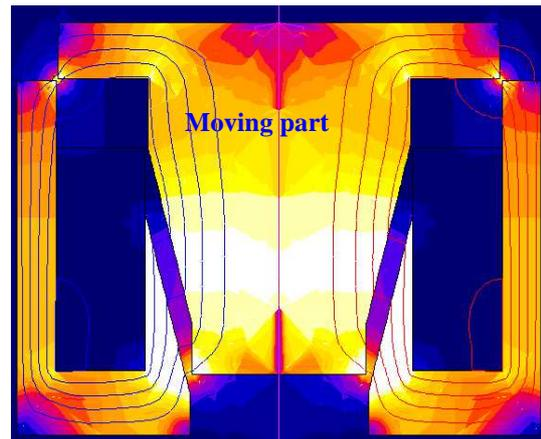
Figure 3. Example of actuator shape that hasn't been chosen: the mobile part is too heavy to suit the application.
