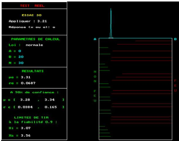
Figure 14. Screenshot showing that all actuations are effective for a 3,5ms long current pulse
