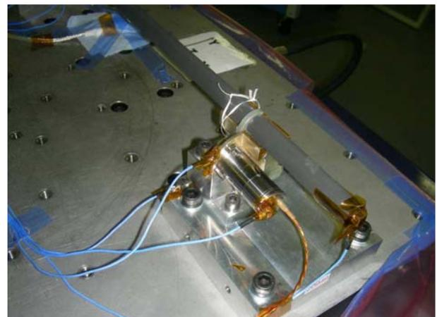
Figure 13. BRUCE integrated to IME-HF antenna for vibration tests
