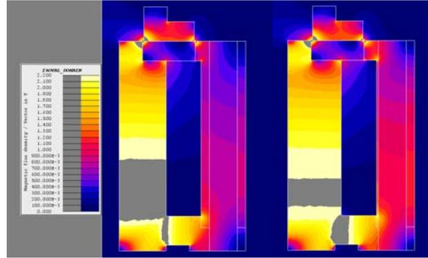
Figure 6. Evolution of the saturation when the coil mean diameter is raised
