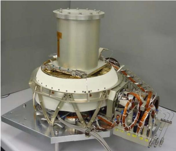
*Figure 8. Thruster Pointing Mechanism (TPM) with Thruster Mass Dummy and Sun-Shield attached.*
