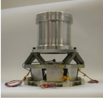
Figure 5. HDRM breadboard for early testing.
