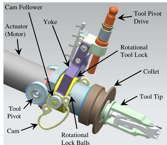
Figure 1 Multifunction Tool Components
