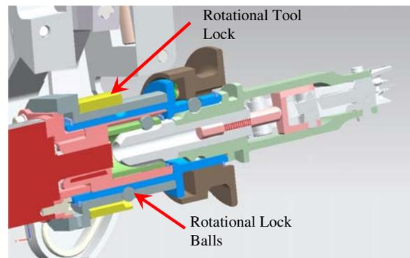
Figure 7 Tool Tip Rotation Lock Mechanism
