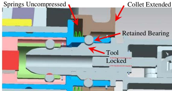
Figure 4 Tool Tip Collet - Locked
