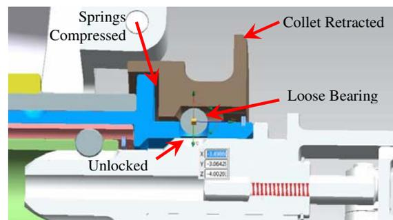
Figure 3 Tool Tip Collet – Unlocked
