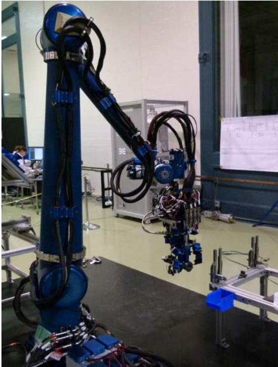
*Figure 14 NGC Manipulator Testing MFT Interface*
