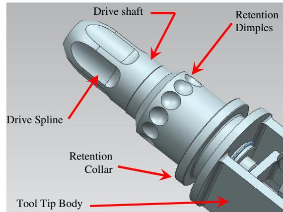
Figure 2 Tool Tip - Interface Elements
