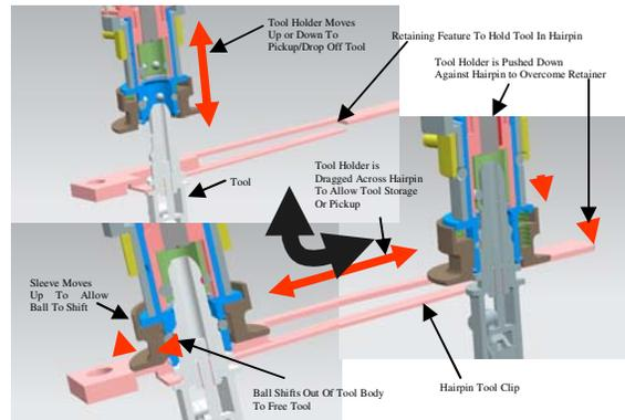
Figure 12 Initial Berthing Holster Operation
