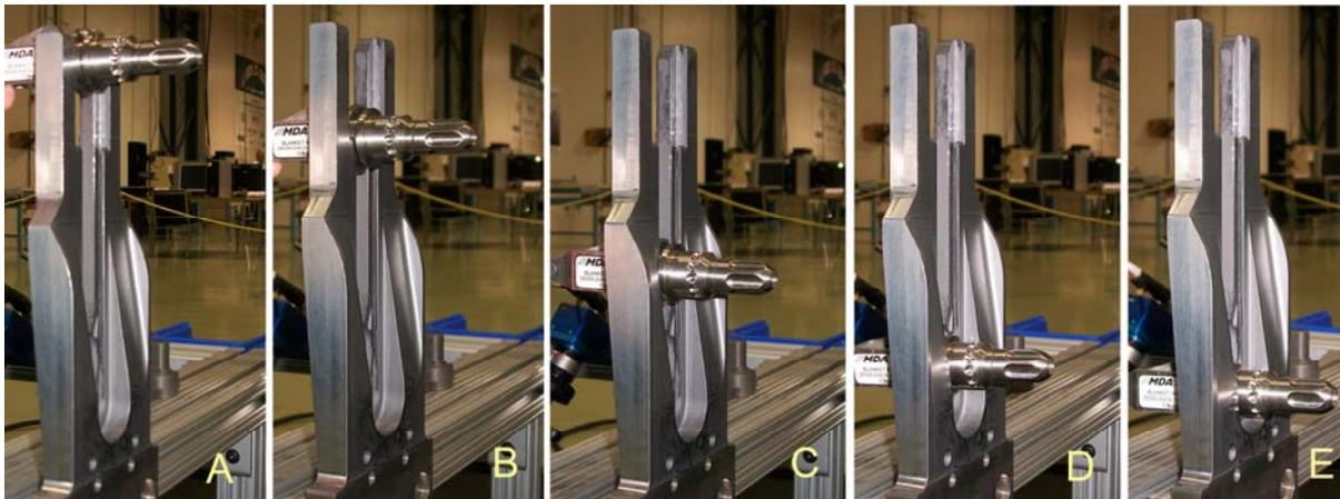
Figure 6 Tool Tip Demate Sequence
