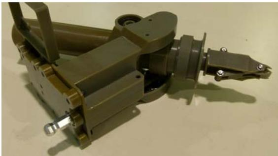
Figure 10 Second Collet Mechanism Prototype
