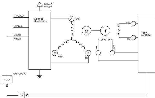
Figure 4. Auto-Ramping with Voltage Controlled Oscillator
