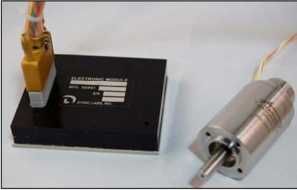
Figure 2. Avior's High Speed Motor and Controller
