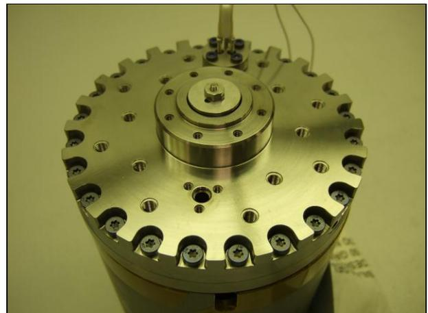
Figure 7. Compressor assembly showing piston in clearance seal.
