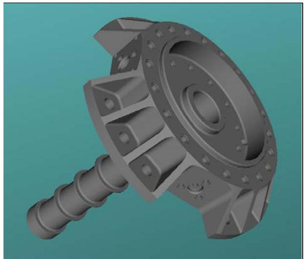
Figure 12. The cold head, showing cold finger stiffening rings and heat transfer ribs at the base
