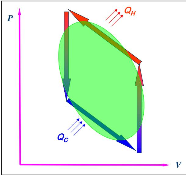
Figure 3. Pressure – Volume diagram of the Stirling Cycle.
