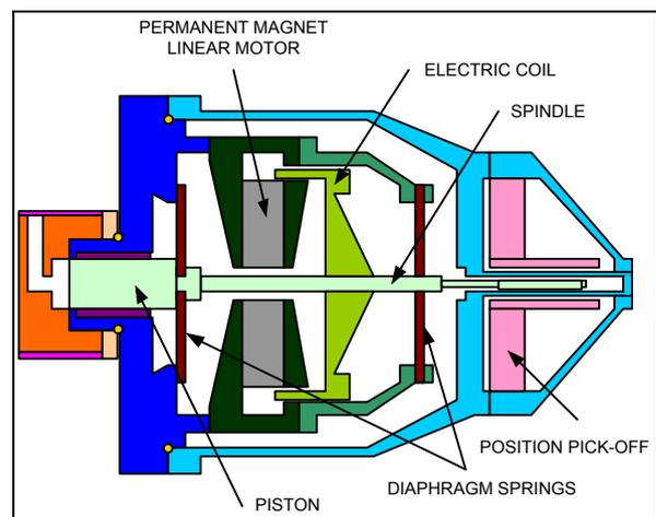
Figure 5. HPSC compressor mechanism.
