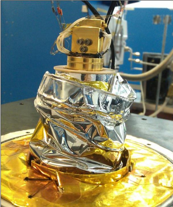
Figure 10. The cold finger fitted with instrumentation and multi-layer insulation
