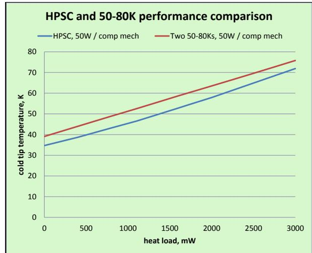
Figure 16. HPSC performance compares to the 50-80K Cooler
