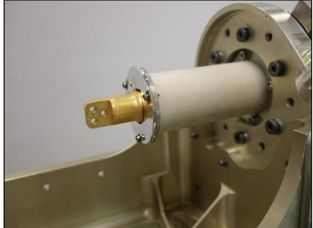
Figure 11. The cold finger snubber of a 50-80K Cooler.
