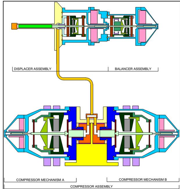
Figure 4. HPSC Schematic.
