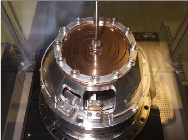
Figure 8. Compressor assembly showing the outer diaphragm spring and lead in wire.
