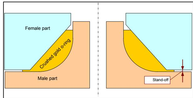
Figure 9. A typical gold o-ring seal geometry.
