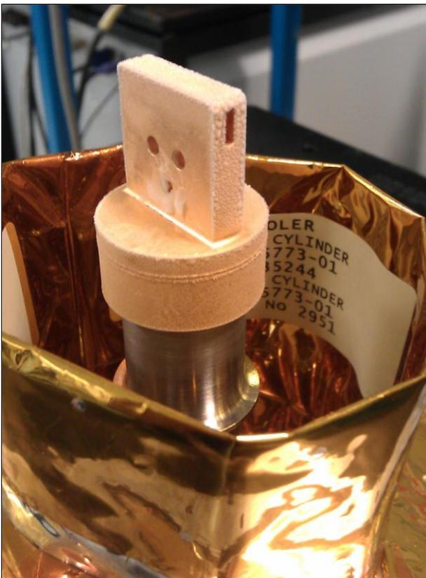
Figure 18. HPSC cold tip showing icing after brief demonstration run in ambient conditions
