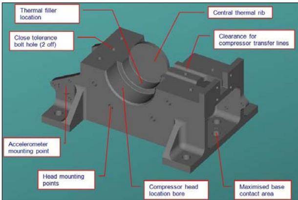
Figure 13. The compressor assembly central bracket lower section with design details shown
