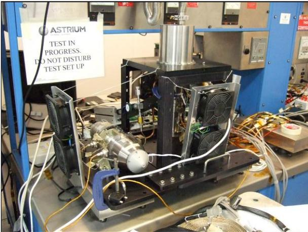
Figure 17. HPSC under life test
