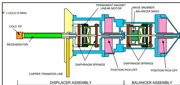
Figure 6. HPSC displacer assembly.
