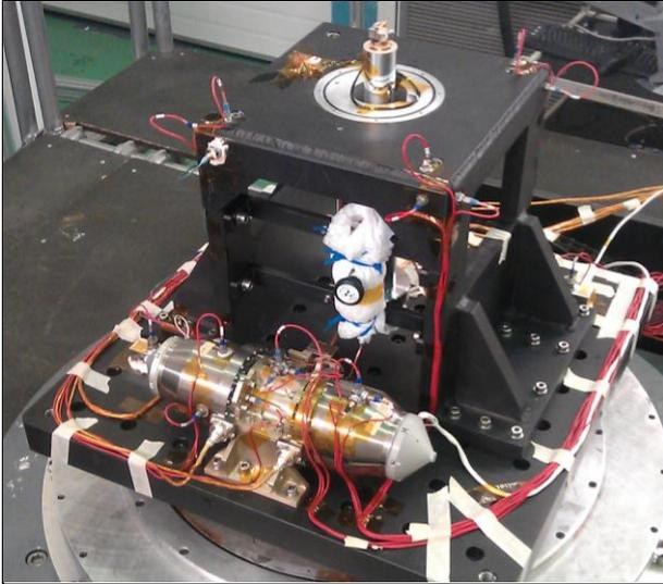
*Figure 1. The High Power Stirling Cooler under vibration test*
