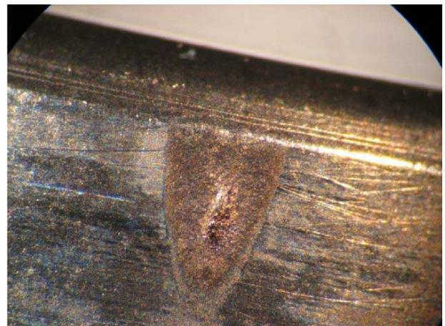
Figure 9. Traces of friction (single bearing outer ring)
