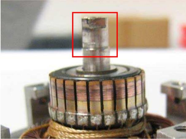
Figure 10. Axial scratches (motor shaft - single bearing location)
