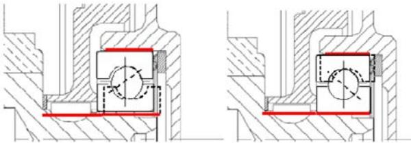
Figure 7. Illustration of sliding of bearing rings
