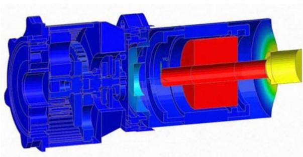
Figure 5. SBGM mode 8 (825 Hz)
