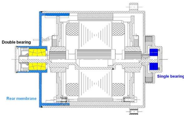
Figure 3. SBGM sealed motor
