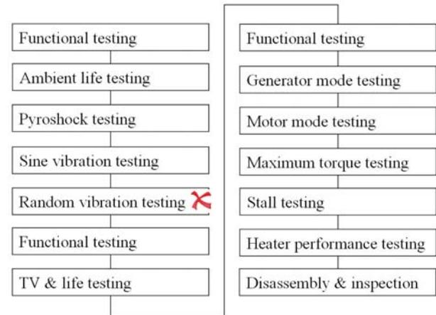
Figure 4. SBGM qualification test flow
