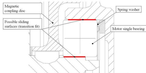
Figure 6. SBGM motor - single bearing configuration
