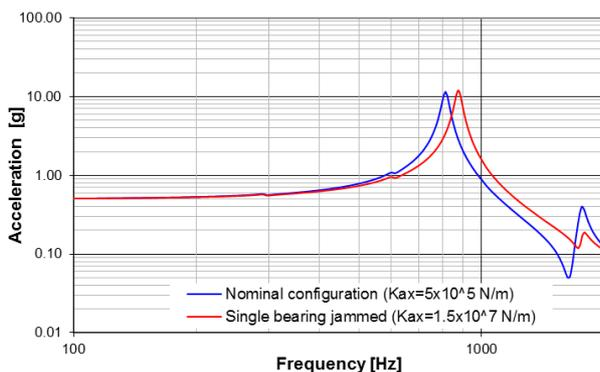
Figure 8. LLS prediction at motor level for Z-axis vibrations - nominal & jammed single bearing
