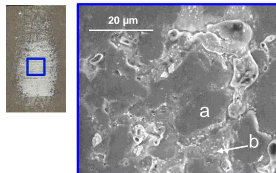
**Figure 7 - SEM image of pad sample from Tecasint 8061 after 3 phase friction test in UHV. a: Polyimide (PI) inclusion; b: isolated 3<sup>rd</sup> body particle.**
