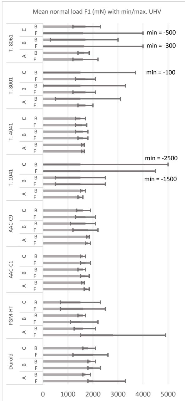
**Figure 2 - Mean F1 load with its min and max (contact retainer/ball) during the friction test in UHV. F = Forward motion and B = Backward motion.**
