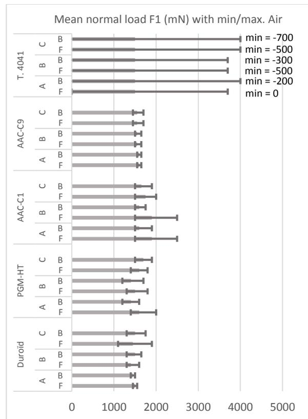
**Figure 8 - Mean F1 load with its min and max (contact retainer/ball) during the friction test in Air. F = Forward motion and B = Backward motion.**
