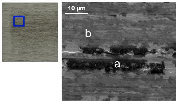
**Figure 5 - SEM image of plate sample from PGM-HT after 3 phase friction test in UHV. a: granular 3<sup>rd</sup> body; b: compacted thin 3<sup>rd</sup> body layer**
