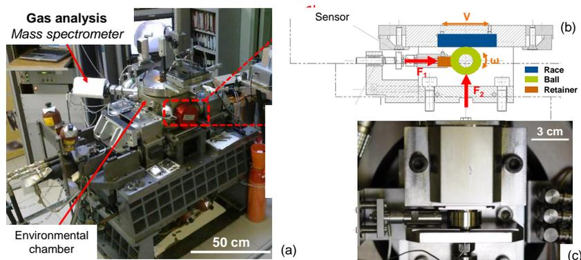
**Figure 1 - Double Transfer Test Bench (DTTB): (a) full tribometer; (b) cross section view of the DTTB ; (c) top view of the contact between the retainer and the ball**
