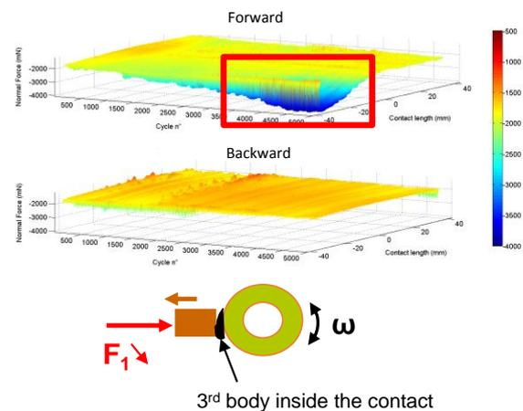
**Figure 3 - Impact of 3<sup>rd</sup> body big particle circulating inside the pad/ball contact: compression of the sensor inducing an increase in the absolute value of the force. Curve from PGM-HT, F1 in mN.**
