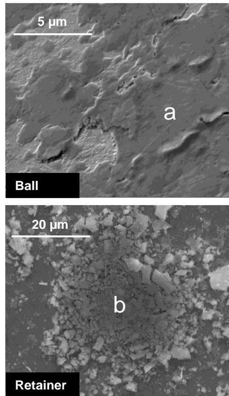
**Figure 6 - SEM images from a ball bearing lubricated with PGM-HT only. a: 3<sup>rd</sup> body layer on the ball; b: 3<sup>rd</sup> body on the retainer at the ball/retainer contact**
