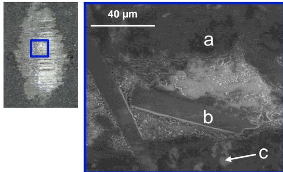
**Figure 4 - SEM image of pad sample from PGM-HT after 3 phase friction test in UHV. a: 3<sup>rd</sup> body (PTFE, MoS<sub>2</sub>, fiber) ; b: fiber ; c: MoS<sub>2</sub>**
