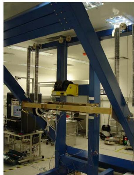
Figure 15. DEM PFM mounted onto functional test fixture with inertia frame
