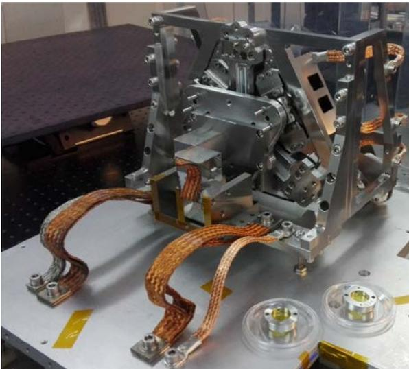
*Figure 19 M2MM ready to install in TV chamber*
