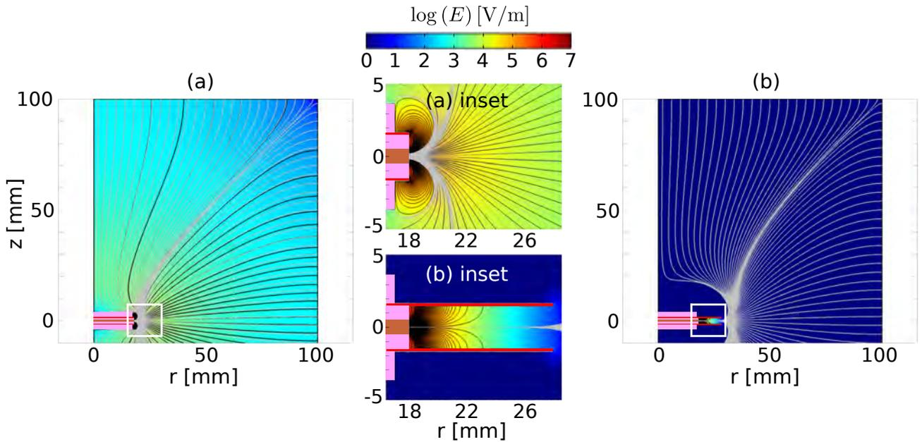
Figure 6. Electric field distribution for (a) the +0 mm, and (b) the +10 mm disc configurations. Detailed views of the corresponding slip ring assemblies are illustrated in the corresponding insets for (a) and (b) marked by the white rectangles. The electric field streamlines leaving the HV-ring surface/chamber wall surface are in black/gray, respectively.
