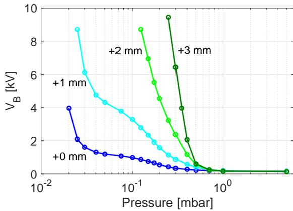
Figure 7. Numerical simulations of breakdown voltage as a function of pressure, for several diameters of the grounded limiting discs.
