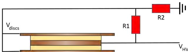
Figure 8. Schematic of a design with passively-biased limiting discs.
