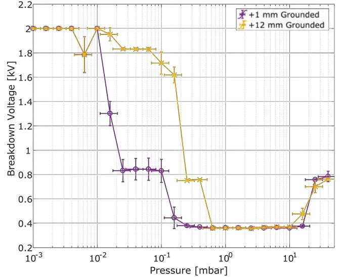
Figure 11. Breakdown curves measured on the advanced SRA mockup for two groups of grounded limiting discs, with a radius exceeding the central HV ring radius by 1 mm and 12 mm.
