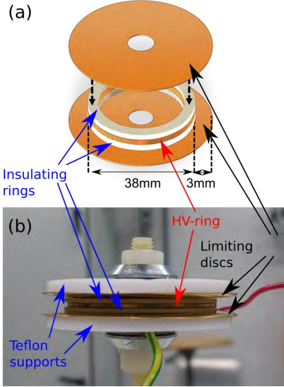
Figure 3. (a) Schematic of the setup. The central HV-ring (yellow) is isolated from the external limiting discs (yellow) by two insulating rings of Vetrinite (white). The top disc is raised to show the lower part of the stack. The insulating support filling the internal volume inside the rings is not shown. (b) Photograph of the assembly.
