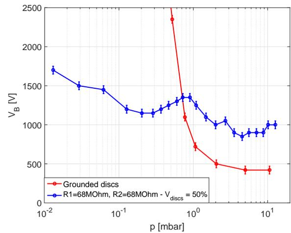
Figure 9. Comparison of breakdown curves for grounded discs (red) and for discs biased to half of the HV-ring voltage (blue).
