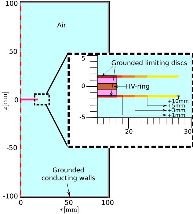
Figure 5. Schematic of the simulation geometry. The vertical dashed red line corresponds to the axis of symmetry. The vacuum chamber walls are indicated in grey. A detailed view of the SRA is depicted. The insulating components are shown in magenta. The grounded limiting discs are in red, with the increasing diameters indicated with different colours up to yellow. The HV-ring is indicated in orange.
