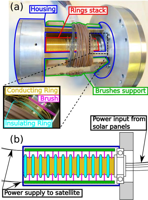
Figure 1. (a) Picture of a cylindrical slip ring for a satellite [5]. The conducting housing surrounding the ring stack is partially removed to expose the slip ring components. A detailed view of gold-plated brushes, gold-plated and insulating rings is shown. (b) Schematic of the slip ring with the colours of the components corresponding to those indicated in (a).
