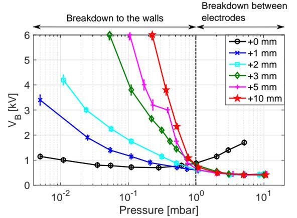
Figure 4. Breakdown voltage as a function of the gas pressure for different grounded discs. The black circles are for the HV-ring alone inside the vacuum chamber. The other measurements refers to the assembly with grounded limiting rings of increasing diameter.
