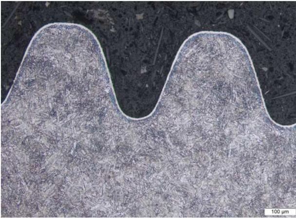
**Figure 4: Microsection of Circular Spline tooth after nitriding**
