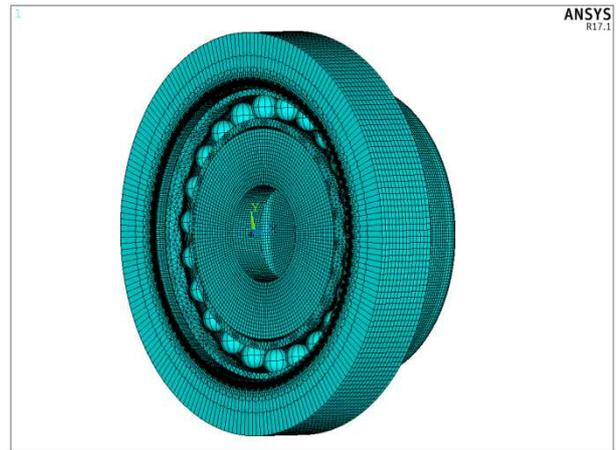
**Figure 8: FE model of a full Harmonic Drive® gear**
