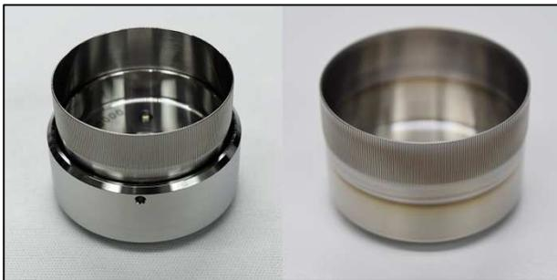
**Figure 5 left: FS prior to nitriding with covering device, right: FS after nitriding**
