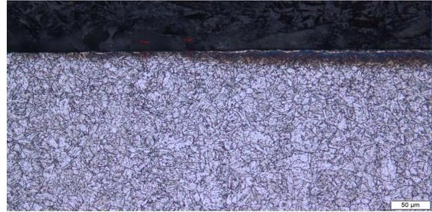
Figure 2: Inhomogeneous nitriding layer on flat sample
