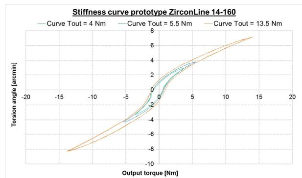
**Figure 10: Stiffness curves prototype**
