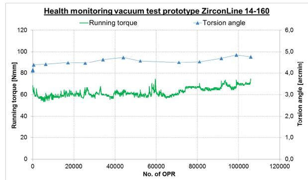
**Figure 11: Results health monitoring vacuum endurance test**
