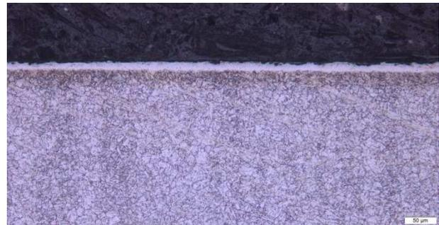
Figure 3: Uniform nitriding layer on flat sample
