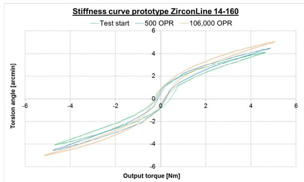
**Figure 12: Stiffness curves measured during vacuum endurance test**
