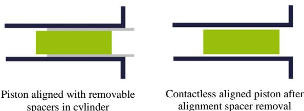
Figure 9: Schematic of motor cylinder with contactless alignment piston.
