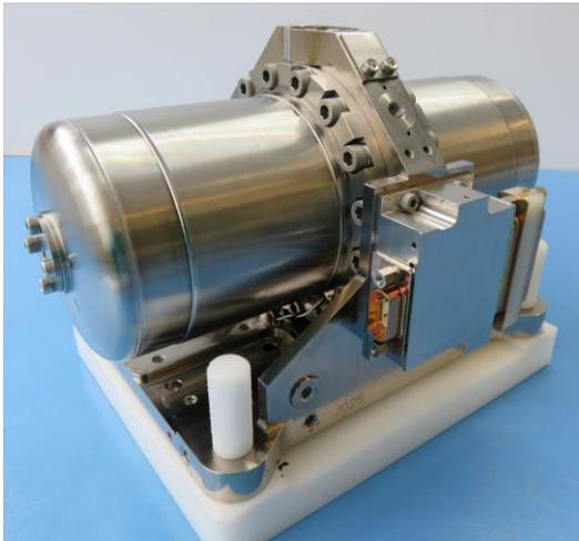
Figure 2: Current compressor Assembly (CPA)
