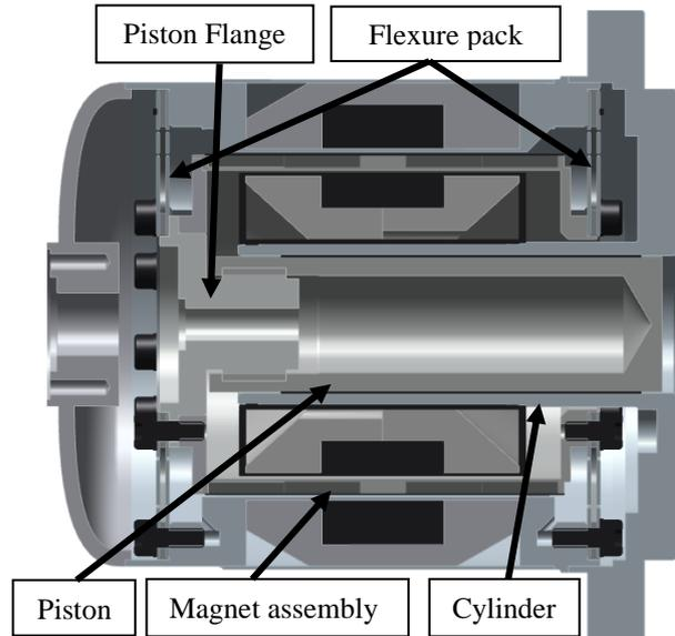
Figure 4: CPA Motor cross-section
