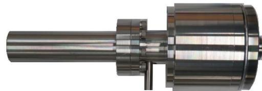
Figure 15: LSF9199/30 Flexure cold finger.
