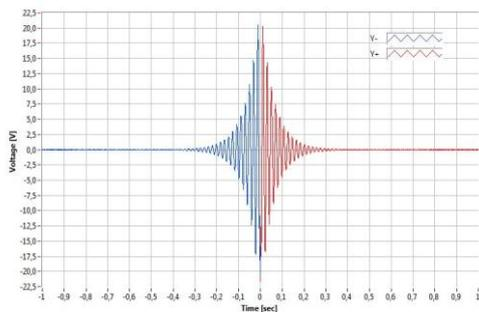
Y-Axes Ring-down at 20°C post environmental test;
