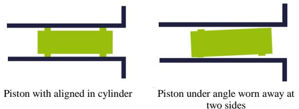
Piston with aligned in cylinder
