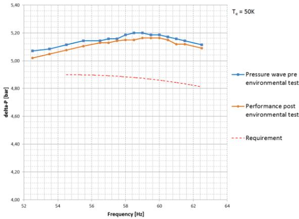
Figure 11: Pressure wave measurement pre and post environmental test
