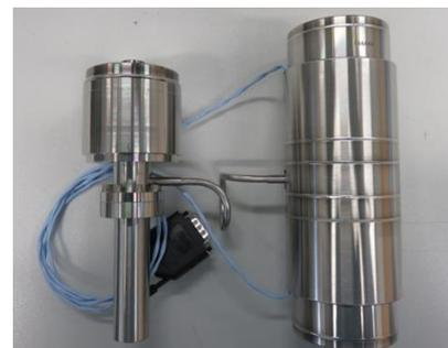
Figure 16: LSF9199/30 Cryocooler
