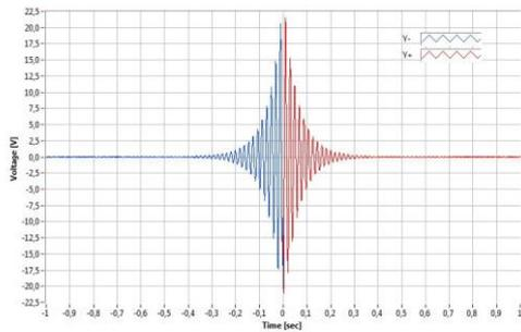
Y-Axes Ring-down at 20°C pre environmental test;
