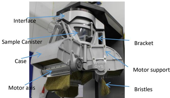
Figure 2. AVS Sampling Tool Mechanism Breadboard
