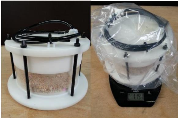
Figure 9. Sample canister full with sampled soil.
