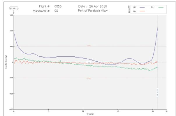
Figure 9. Example of flight microgravity phase profile
