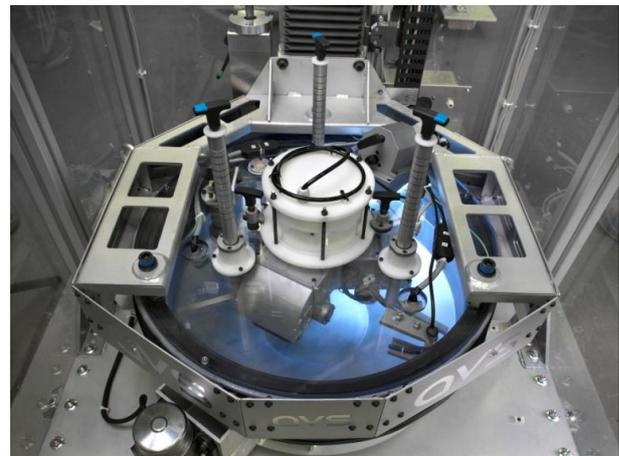
Figure 4. Experiment rack 1: Motorized sampling tool and regolith simulant container
