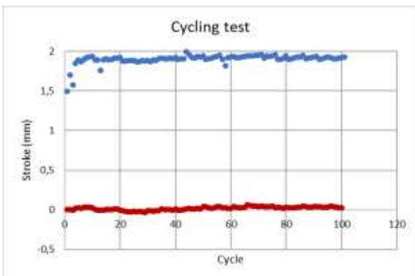
Figure 7: Cycling test. Red and blue curves show triggered and reset position
