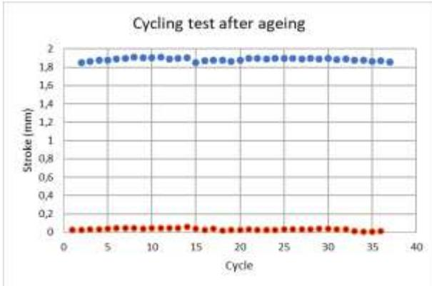
Figure 10: Cycling test after 120°C ageing
