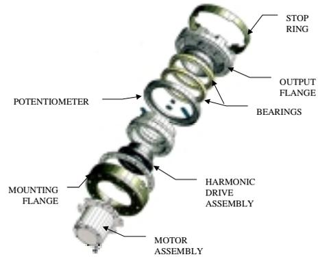
**Figure 2: PTAG Actuator Assembly**
