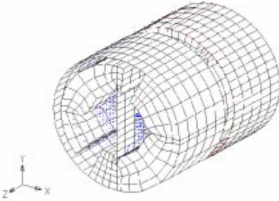
The figure hereafter shows only the blades, modeled with SHELL elements.
