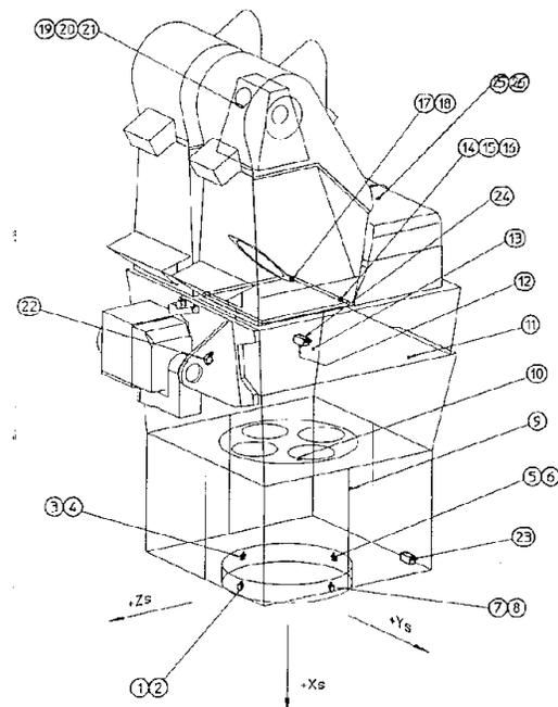
22 : one accelerometer near the PASTEL telescope
