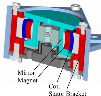
Fig.: 6-1 Diagonal cut through the FPA
