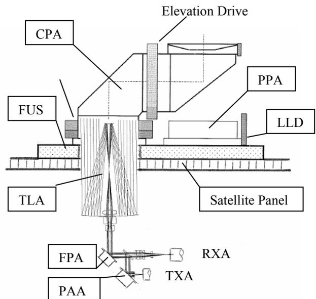
Fig.: 3-1 Functional Arrangement of the PAT Mechanisms
