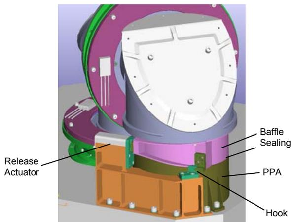
Fig.: 5-12 Arrangement of LLD Actuator
