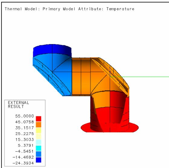
Fig.: 5-6 Temperature distribution in Cold Case (hot FUS I/F)
