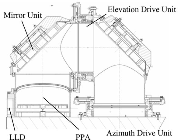
Fig.: 5-2 Cross Section through CPA
