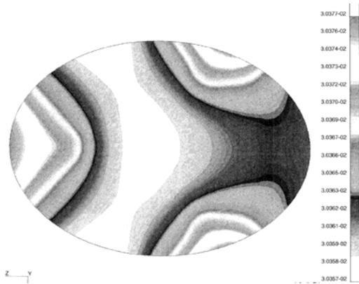
Fig.: 5-11 RMS error caused by Mirror Attachment Interface with integrated SIC bolt
