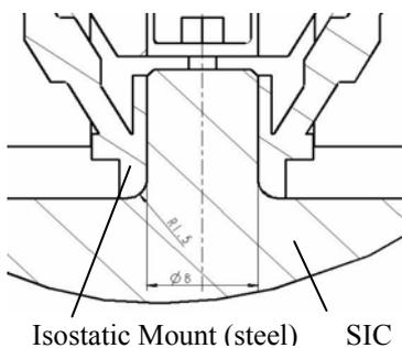
Fig.: 5-10 Improved Attachment Interface between Mirror and Isostatic Mount
