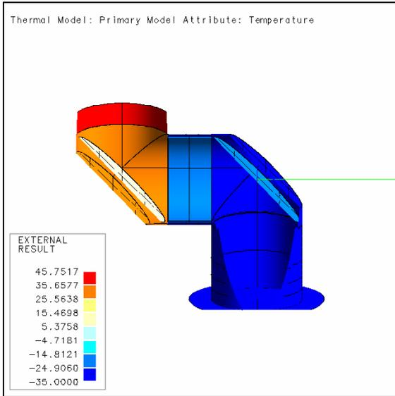
Fig.: 5-5 Temperature distribution in Hot Case (cold FUS I/F)
