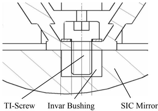
Fig.: 5-8 Mirror Attachment Interface (Invar Bushing)
