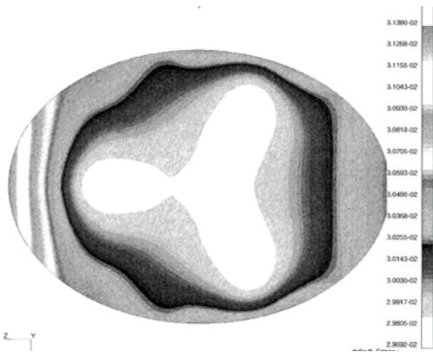
Fig.: 5-9 RMS error caused by Mirror Attachment Interface with Invar bushing
