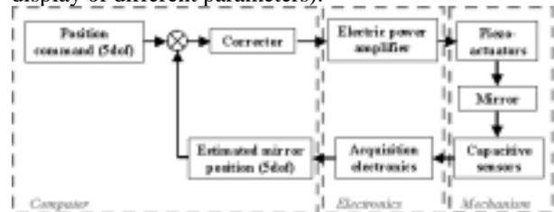
Figure 6 : Closed loop of mechanism control
