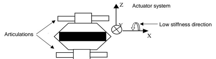
The mechanism's rotation plan is located 40 mm under the mirror inferior plan.
