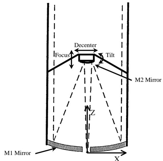
Figure 1 : Definition of the geometrical instabilities
