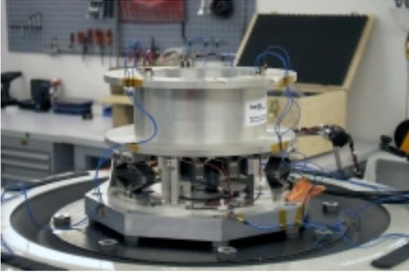
Figure 9 : MCM during the Z vibrations test
