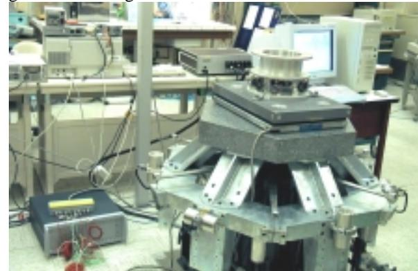
Figure 10 : the lay out for the microvibrations tests
