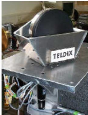
Figure 3: CMG momentum wheel under lifetime tests at Teldix
