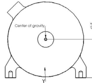
**Fig III : Localisation of the center of gravity following Y axis**
