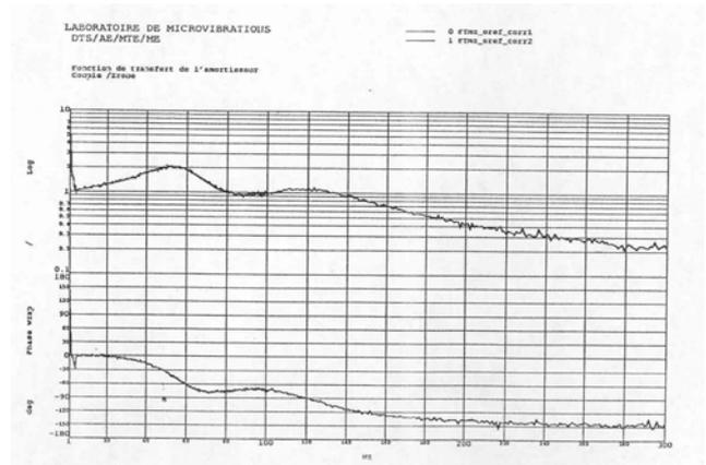
**Fig XV : Torque transmissibility**
