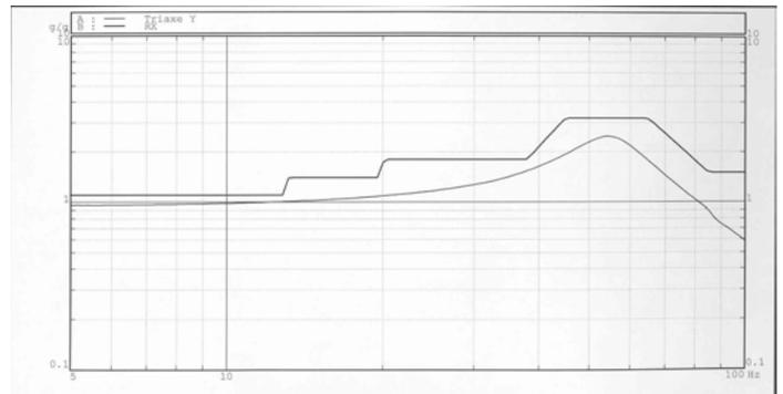
**Fig XII : Transmissibility following Y axis (factory acceptance test at 25°C)**
