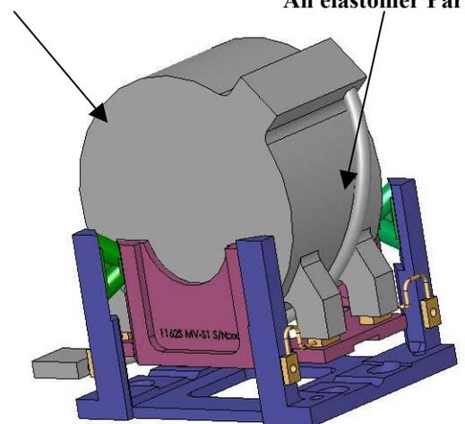
**Fig IV : the damping isolator system and its reaction wheel**
