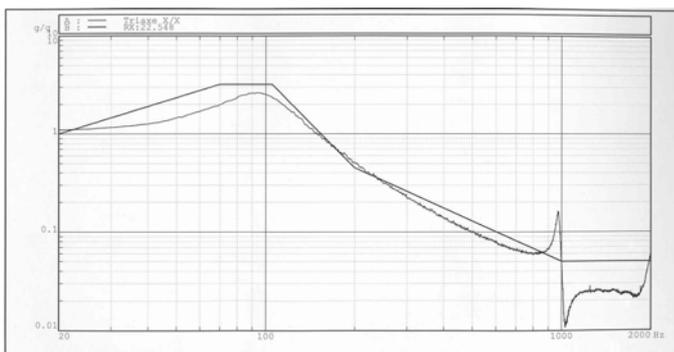
**Fig XI : Transmissibility following X axis (factory acceptance test at 25°C)**
