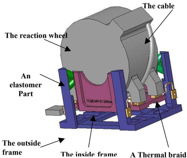
**Fig X : The damping isolator system and its reaction wheel**
