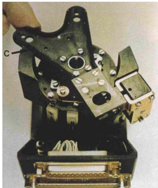
Fig. 1 Mechanism of a satellite: anchor was actuated from its resting position (middle) electromagnetically. It impacted on both end stops. Finally, an anomaly from the satellite was reported, that the anchor kept blocked on the left side. It was “cold welded”.
