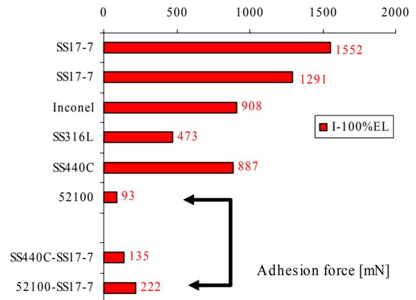
Fig.5 Adhesion force under impact for different types of steel versus itself: austenitic structure and Ni seem to promote high adhesion: SS17-7ph (7%), AISI 316L (11%), Inconel 718 (52%). No adhesion for AISI52100 versus itself (“52100”). High adhesion of AISI440C has to be proven. Combinations of different steels: adhesion seems to increase in contact to steels with higher tendency to cold welding (arrow).
