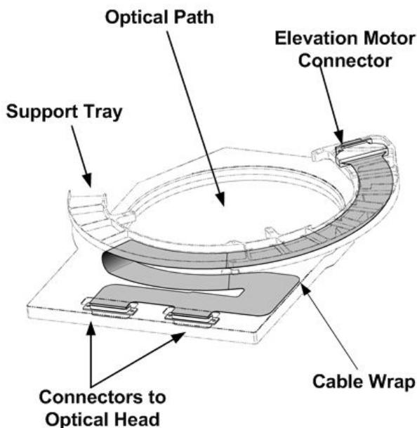
**Figure 12. Omega Cable Wrap**
