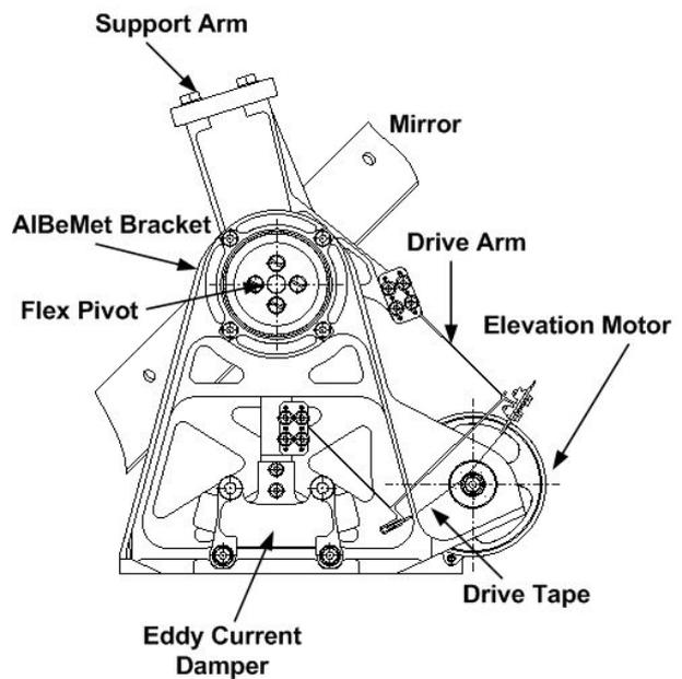
**Figure 3. Elevation drive system**
