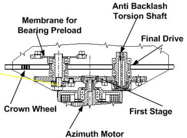
**Figure 11. Cross Section of Gearbox**
