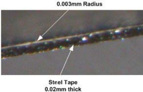
**Figure 4. View on edge of Steel Tape**
