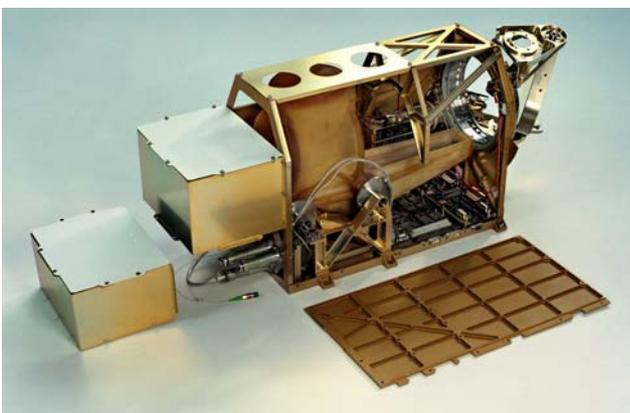
Figure 1. Photo of the Breadboard ISLFE OH
