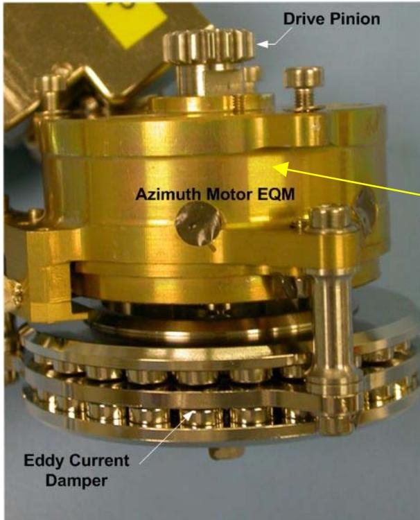
**Figure 9 Azimuth Damper**
