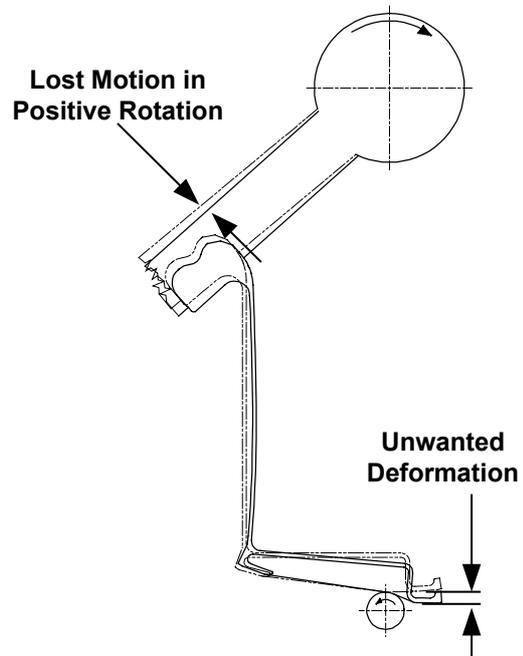
**Figure 6. Local Deformation of Elevation Arm**
