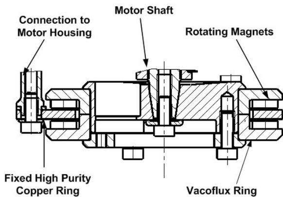
**Figure 10. Cross Section of Azimuth Damper**
