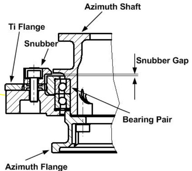
**Figure 8. Azimuth Bearing Installation**
