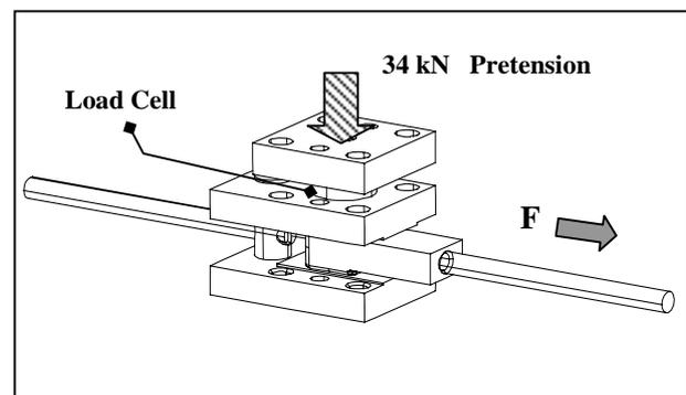
Figure 3 – Test Set-up for measuring friction coefficient
