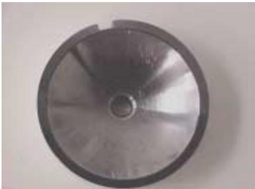
Figure 13 – Upper Fitting after 200 Cycles
