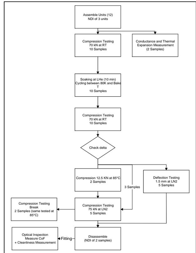
Figure 6 – Qualification testing of interface struts
