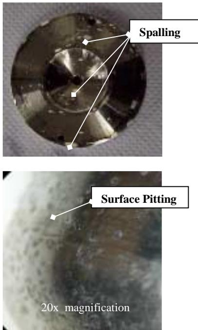
Figure 8 – Corrosion of MoS<sub>2</sub> Coating
