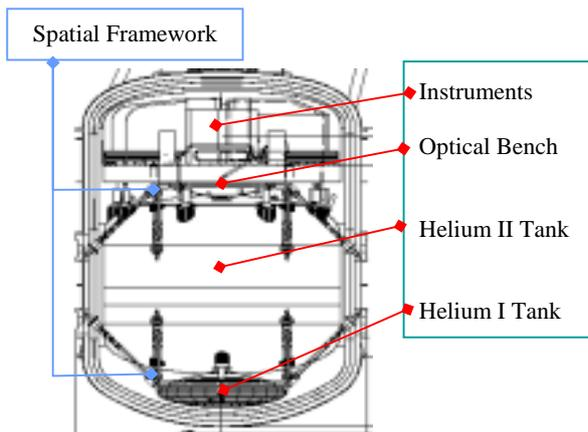
Figure 1- Location of Spatial Framework in the cryostat
