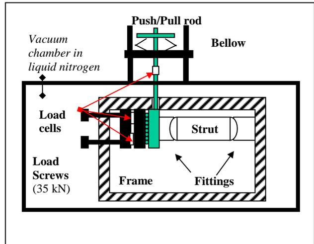
Figure 10- Test schematic for cryogenic testing under vacuum
