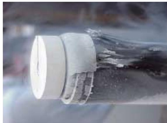
Figure 7 – Compression failure of unit at 77 K
