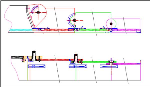
**Figure 7:** guides and latches in the deployed configuration
