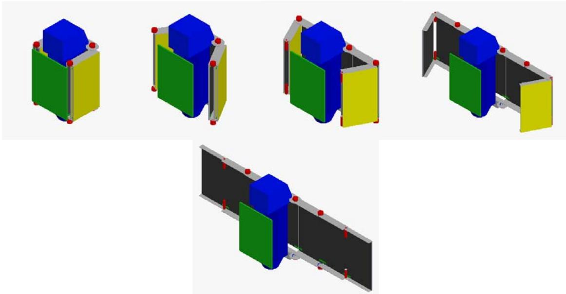
**Figure 1:** Antenna deployment sequence
