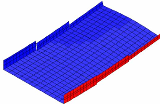
**Figure 5:** first vibration mode of the deployed antenna
