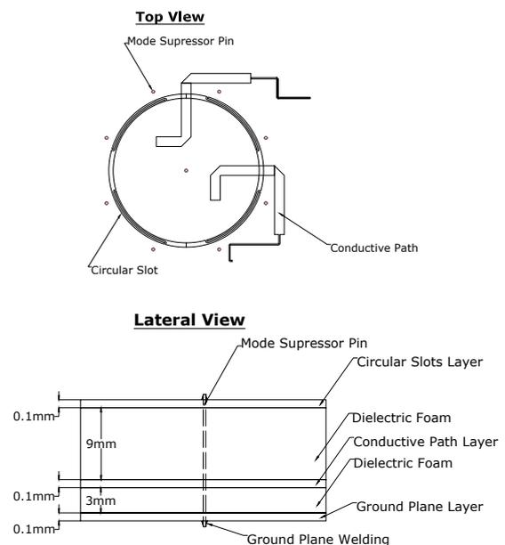
**Figure2:** radiating structure scheme
