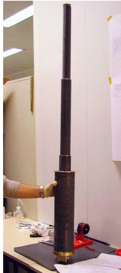
Figure 8: Engineering model first & second tube deployed
