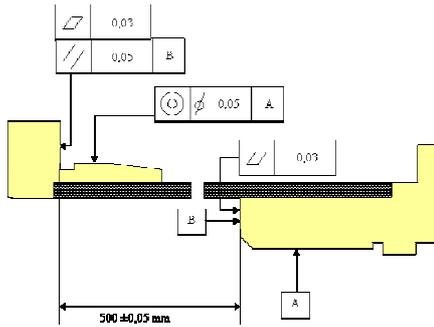
Figure 7: Geometric tolerances between both end rings
