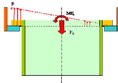
Figure 4: Schematic representation of junction with planar contact
