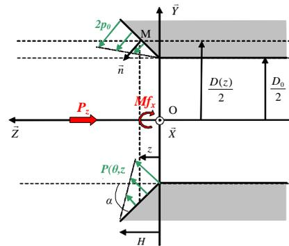
Figure 3 : Schematic representation of conical assembly
