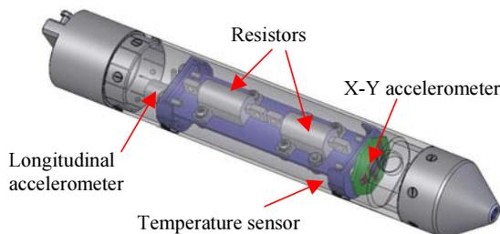
Figure 6 Trailed Mole dummy model
