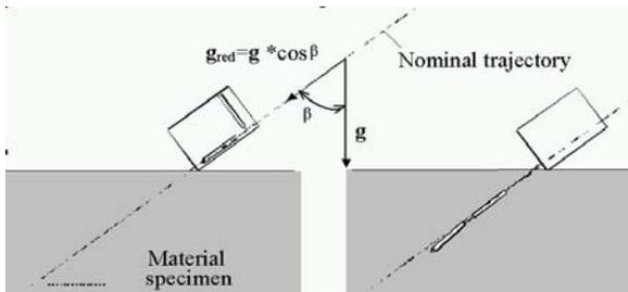
Figure 12 Simulated reduced gravity test
