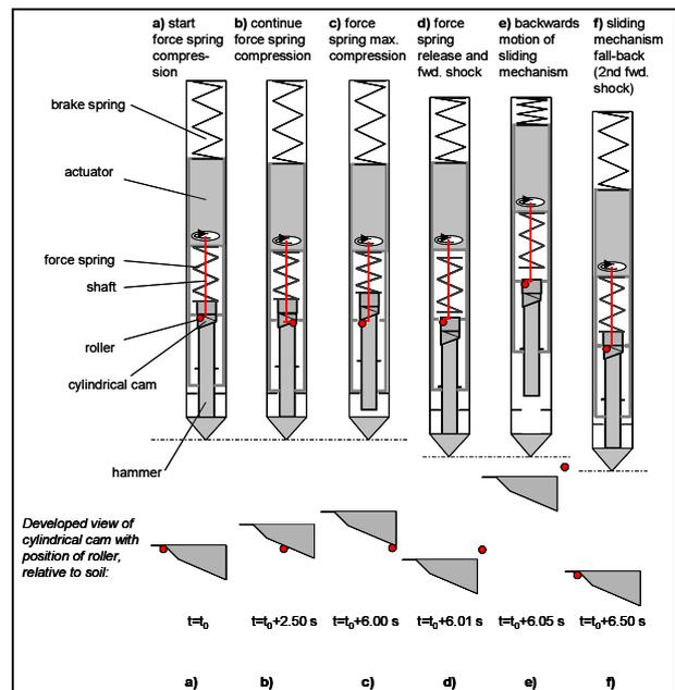
Figure 5 Schematics of hammering mechanism sequence during a single shock cycle
