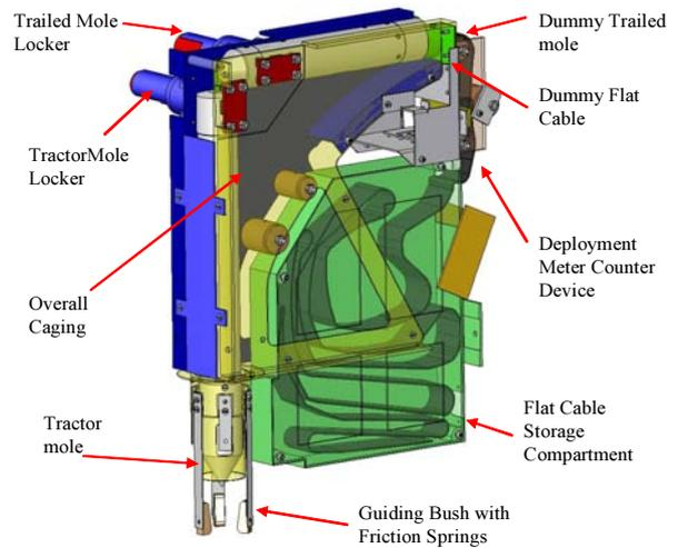
Figure 2: IMS overall view (305 x 238 x 112 mm)
