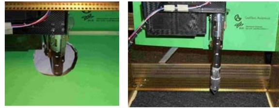
Figure 15 The tractor mole in the soil at the end of the test (left) and extracted from the soil (right)
