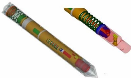
Figure 4 Exploded views of the Tractor Mole
