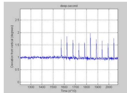
Figure 11 Noise on vertical angle measurement
