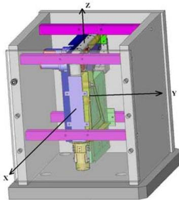
Figure 14 Vibration tests reference axes
