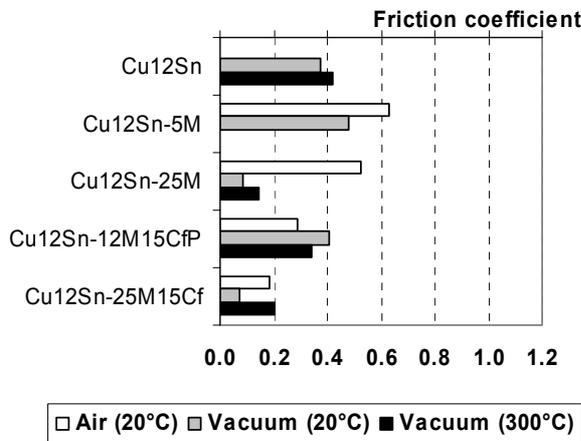
Figure 4: Friction coefficient of Cu-MMCs (cp-process) in air, vacuum and Vacuum/300°C. Best composition for "all environments is Cu12Sn-25M15Cf.
