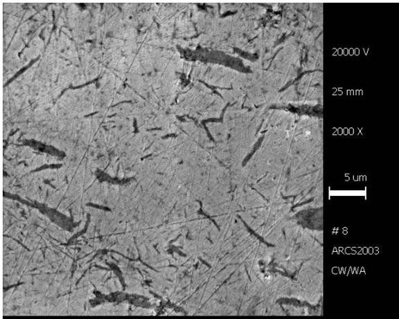
Figure 2: SEM image: dense metal matrix with well distributed MoS<sub>2</sub> particles (dark).
