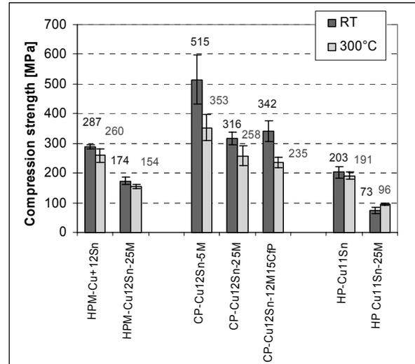
Figure 3: Compression properties of Cu-MMCs: compression strength (elastic limit) the high filled CuMMCs (~25v% fillers) by the ARC-cp-route show higher values than hp- and hpm-MMCs.
