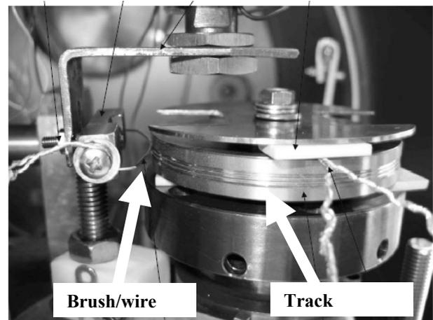
Figure 1: Slip-Ring test setup in vacuum tribometer
