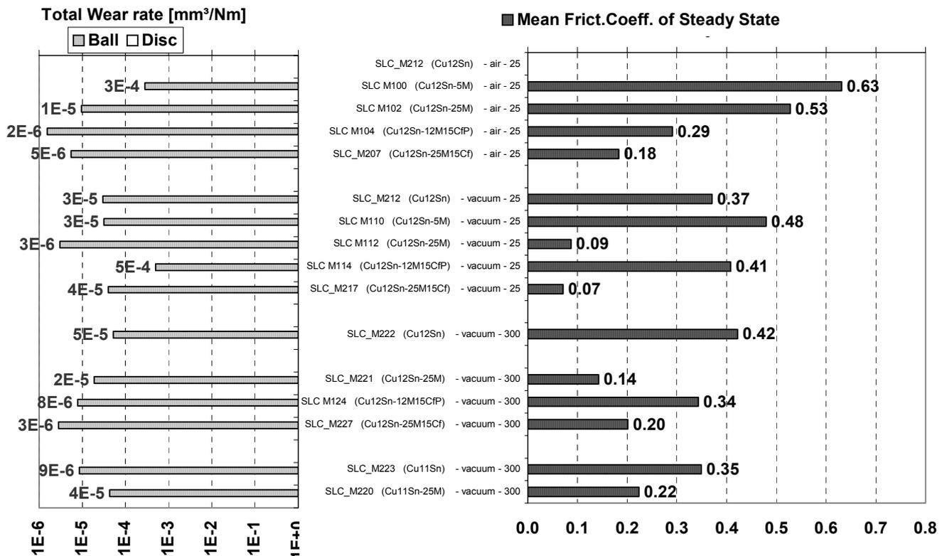
Figure A1: Survey of Friction coefficient and wear rate in air (50%rH) and vacuum: applied loads achieving 2/3Ys of each Cu-MMC. Air: Lowest friction achieved by carbon fibres. Vacuum: lowest friction achieved with only higher amounts of MoS<sub>2</sub>(25v%). Combination of MoS<sub>2</sub> and carbon fibres successful: low friction in both air and vacuum (←). Reference material Cu11Sn-25M comparable reason
