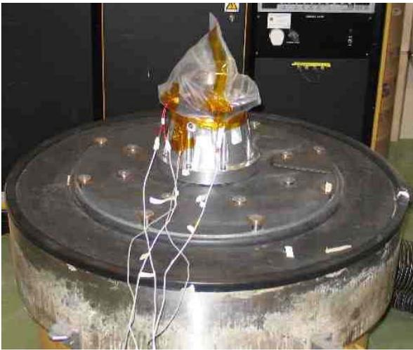
Figure 15. APM Breadboard bagged on vibration shaker.
