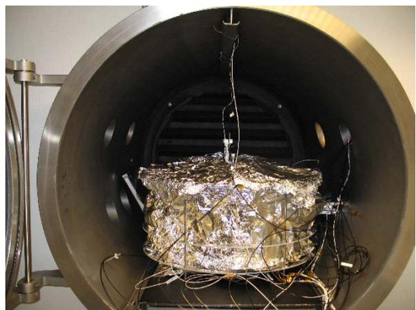
Figure 13. APM Breadboard isolated by aluminum foil in vacuum chamber.
