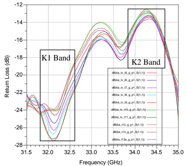
Figure 9 Effect of Temperature on Ka-band Return Loss
