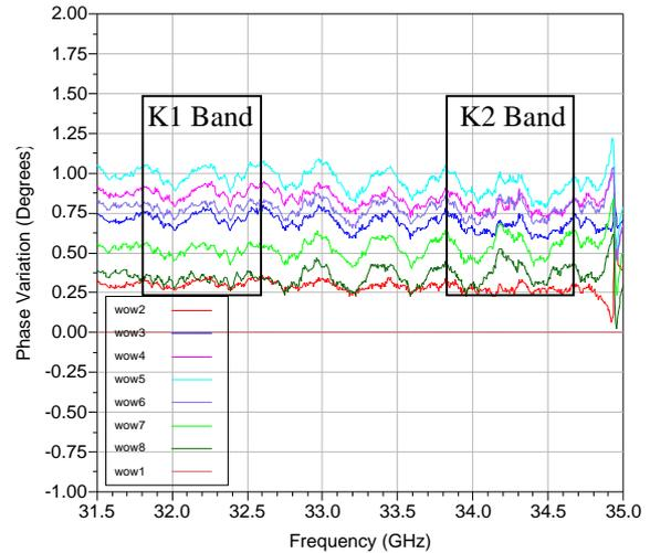
Figure 11. Wide-band Plot of Ka-band Relative Transmission Phase for 360° of Rotation at 240°C
