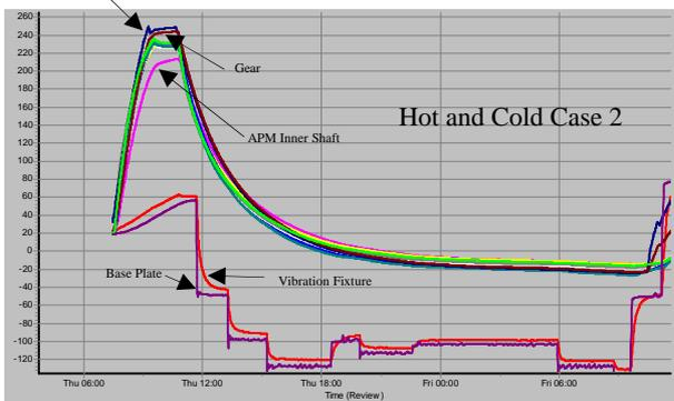
Figure 14. Temperature curves for Hot and Cold case.
