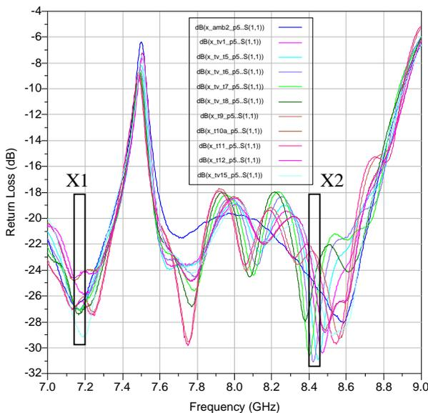
Figure 8 Effect of Temperature on X-band Return Loss Compared to Ambient Non-chamber Plot
