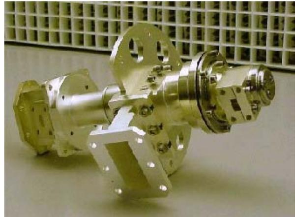
Figure 1. RF Rotary Joint.
