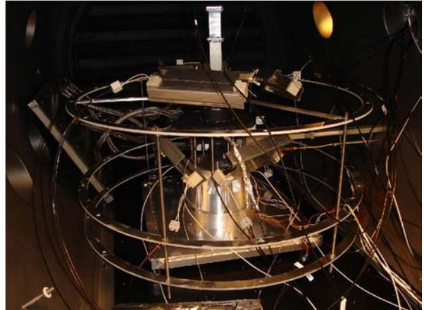
Figure 12. APM Breadboard with IR lamps and RF connections in vacuum chamber.
