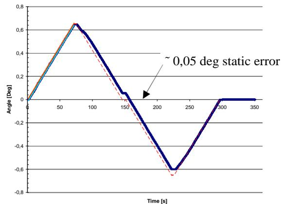
Figure 4. APM pointing performance (blue curve is measured shaft position, red is theoretical by commanded motor steps).
