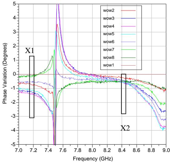
Figure 10. Wideband Plot of X-band Relative Transmission Phase Variation for 360° of Rotation at 240°C
