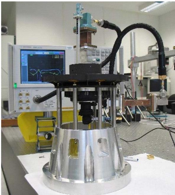
Figure 7. APM during RF functional test in air.
