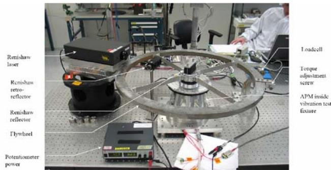
Figure 6. APM Functional Test.
