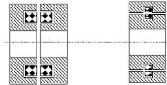
Figure 1 : standard transformers (axial or radial gap)
