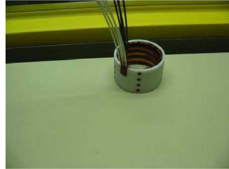
figure 16 : Transformer coils glued in housing
