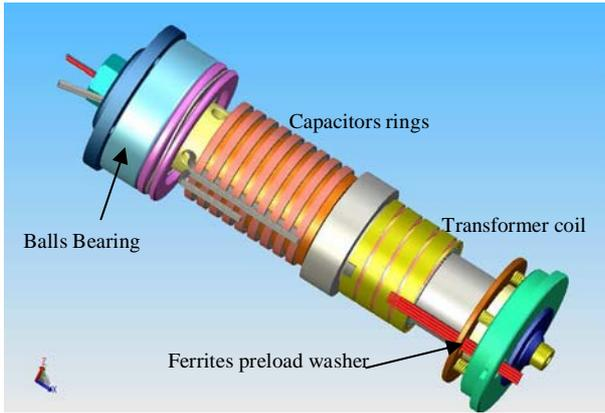
figure 19: Slip ring internal view
