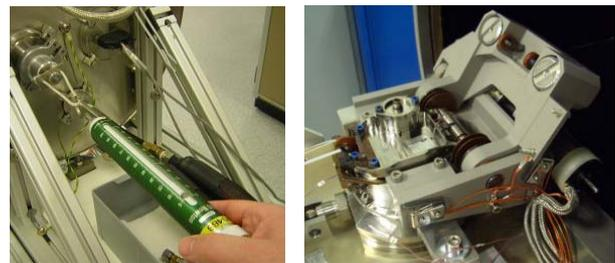
Figure 12: Test setup for motorization margin tests with Spring Gauge outside and LOM with CGSE inside the vacuum chamber
