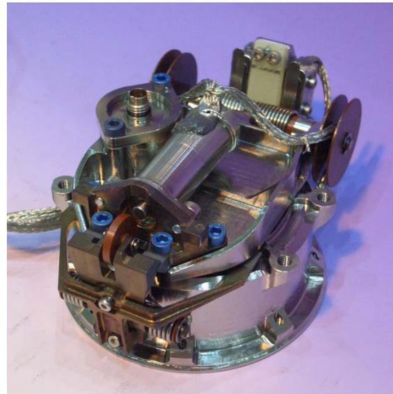
Figure 14: LOM in closed configuration (diameter 80mm, height 50mm)
