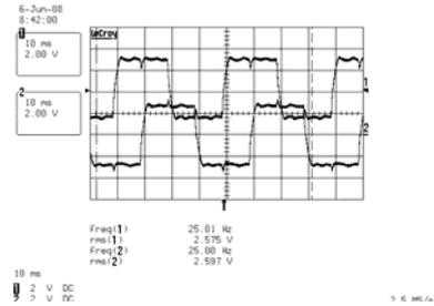
Figure 11 Motor current = 103 mA Step rate 100pps
