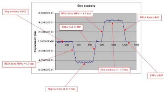
Figure 17 Displacement measurement during "Accuracy test" at AT
