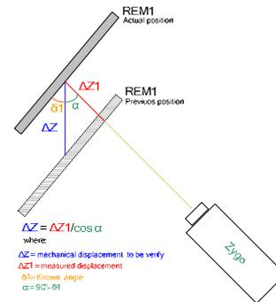
Figure 16 Set-up for displacement measurement in TVC
