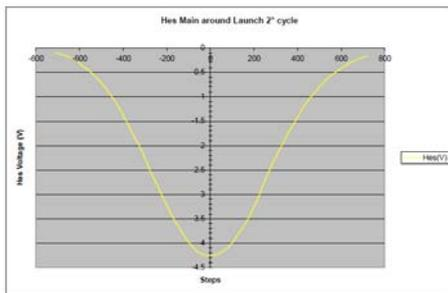
Figure 12 HES signal (main) around Launch position at mOT
