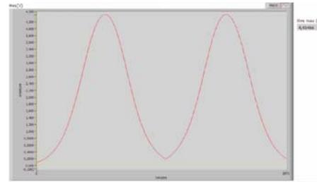
Figure 14 HES signal (main) around mid-stroke position at mOT (two acquisitions)
