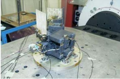
Figure 26 RMA LTM on the vibration table
