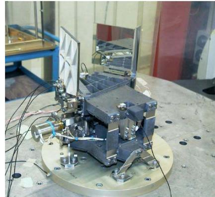
Figure 5 RMA AQM on the vibration table
