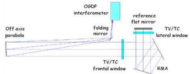
Figure 25 WFE test set-up at cryogenic temperature
