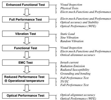
Figure 3 NIRSpec RMA qualification test sequence
