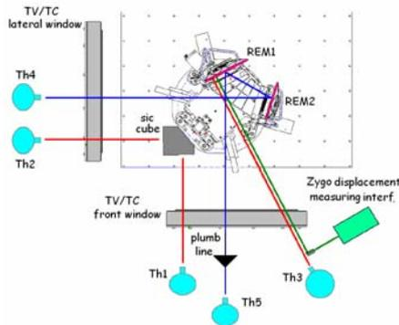
Figure 24 Alignment verification set-up for TV cycling
