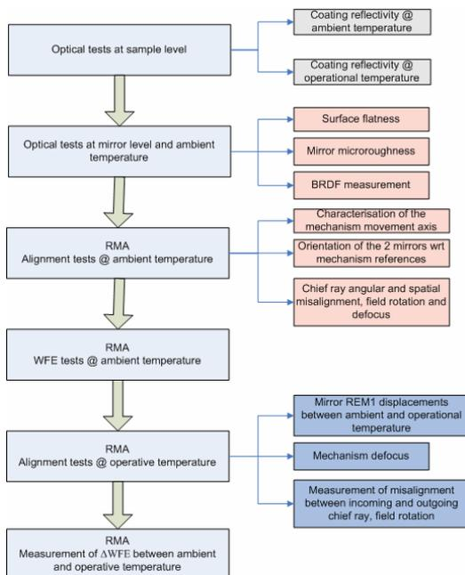
Figure 21 Optical tests at sample, mirror and RMA level
