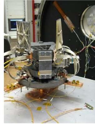
Figure 8 AQM TV/TC set-up
