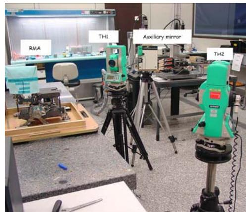
Figure 22 Alignment verification at AT
