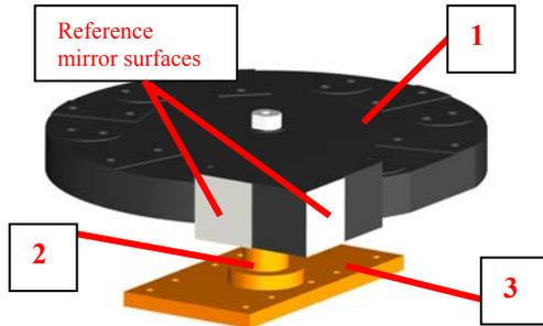
Figure 6 TV/TC mechanical interface
