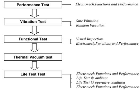
Figure 4 NIRSpec RMA Life Model test sequence
