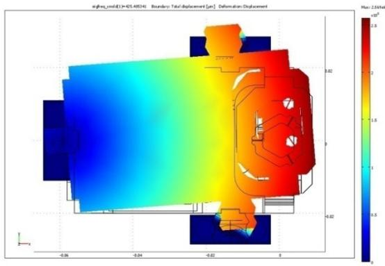
Figure 14. The first eigenfrequency at 425 Hz
