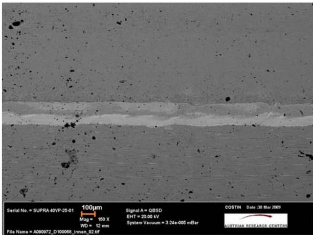
Figure 7: SEM-image (Back-scattered mode): Inner race with transfer layer taken from bearing run at vacuum 300°C (bright track in middle).
