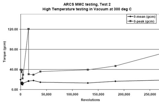
Figure 3-3: Test results in vacuum at 300 deg C
