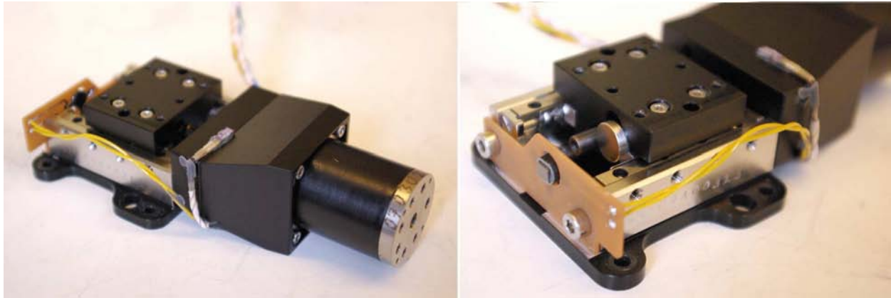
Figure 3 Views of QM mechanism and details on end of course sensor and roller cages
