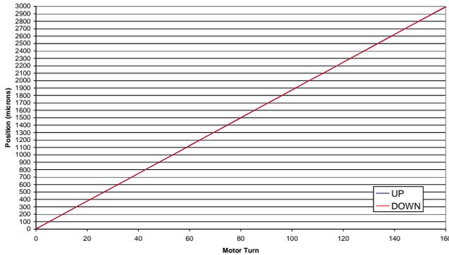
Figure 17.- 160 motor turns (up and down direction).
