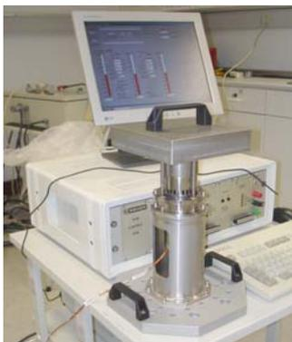
Figure 14.- Torque margin set-up
