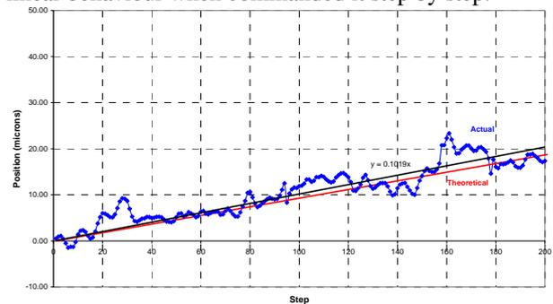
Figure 16.- Motor step by step linear advance.
