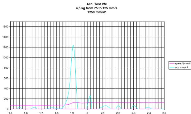
Figure 4 Acceleration profile on the VM actuator
