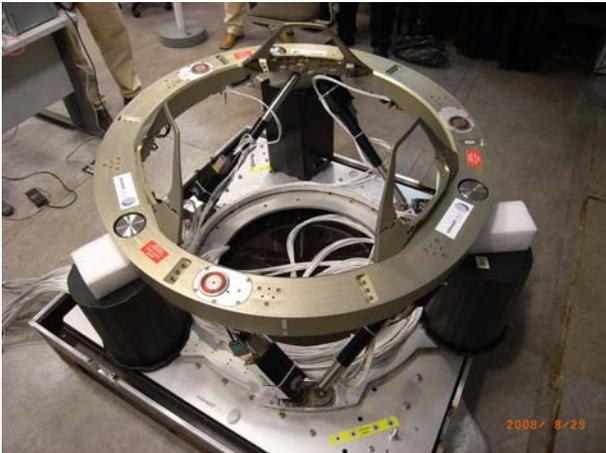
Figure 14 IBDM actuators in the IBDM Hexapod
