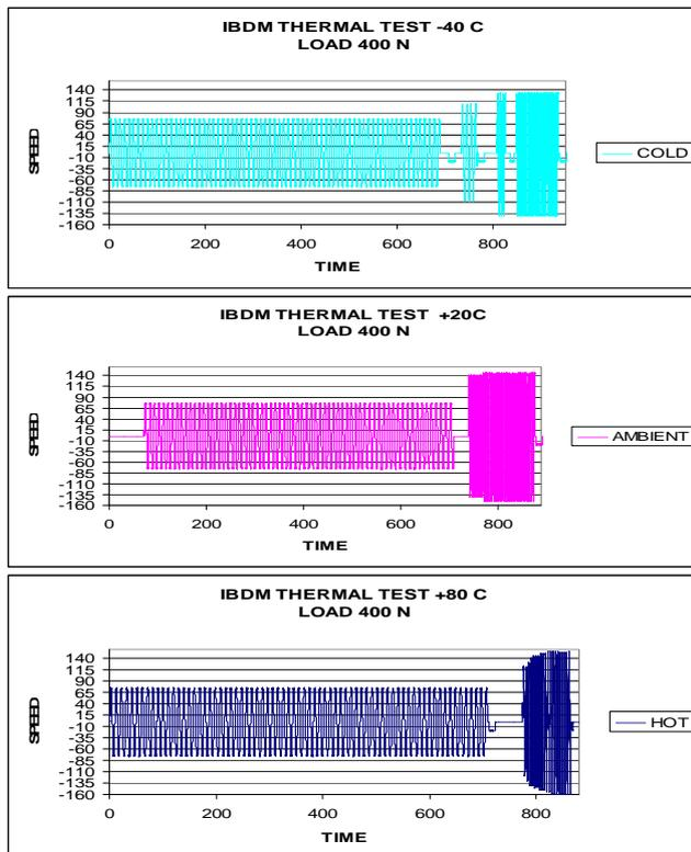
Figure 11 VM actuator life cycles during TV test
