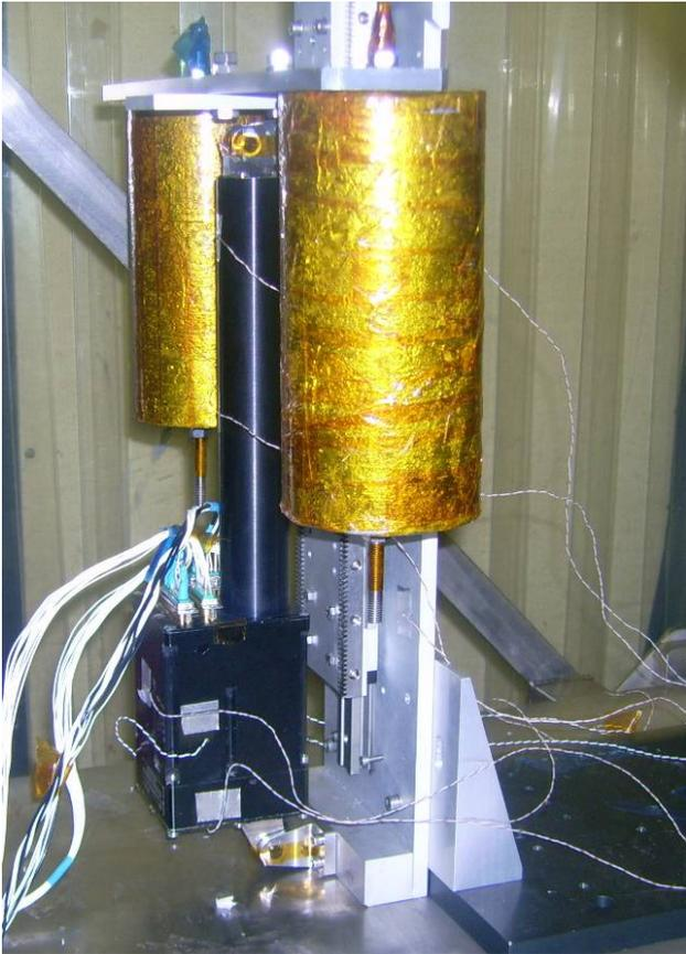
Figure 10 VM actuator in TV test configuration
