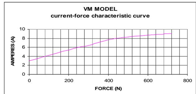
Figure 2 Current- force curve for VM actuator
