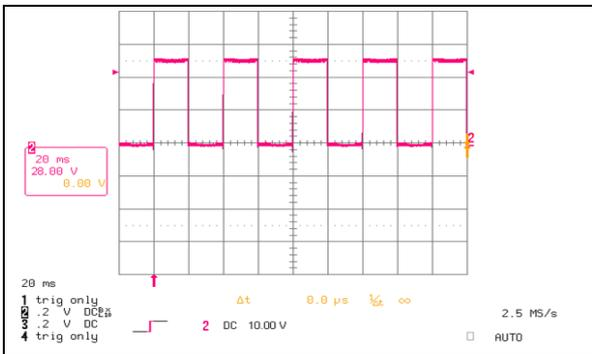
Figure 5-3 Driver Signal Pulses.
