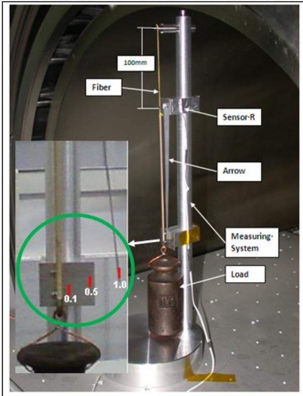
Figure 4-8 Measuring System.
