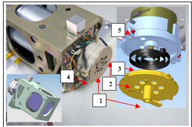
Figure 2-1 The MPOI and EPA Module.
