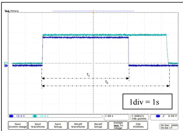
Figure 4-5 Fiber time burn at -30°C.
