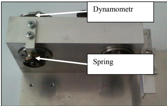
*Figure 5-7 The spring measurement system.*
