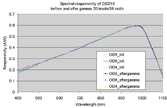
Figure 14. Photodiode sensitivity drift due to ionizing dose
