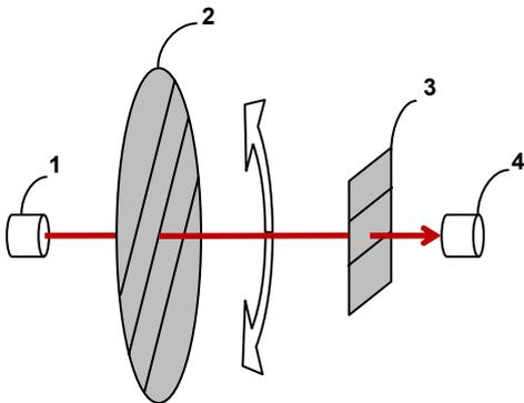
Figure 3. Modulation of illumination by two polarizers
