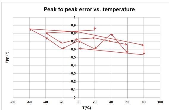
Figure 11. Evolution of encoder's accuracy during thermal cycling
