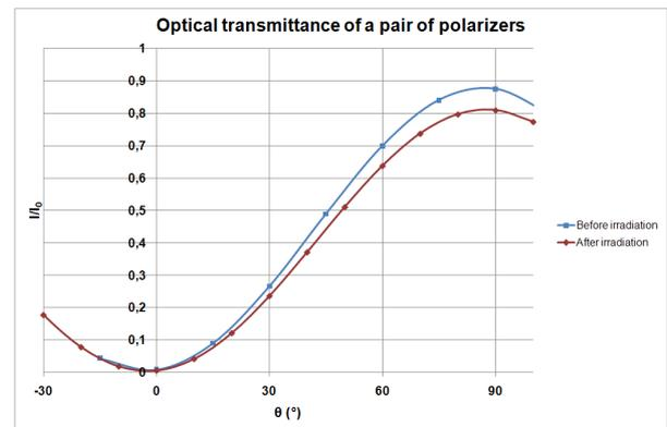
Figure 13. Optical transmittance measurements before and after irradiation
