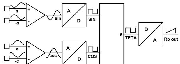
Figure 5. Signal shaping and processing
