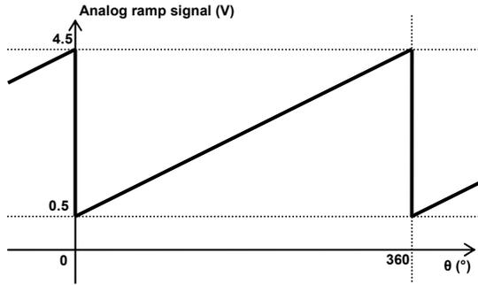
Figure 1. Output for a full analog ramp over 360°
