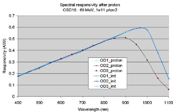
Figure 15. Photodiode sensitivity drift due to displacement damage
