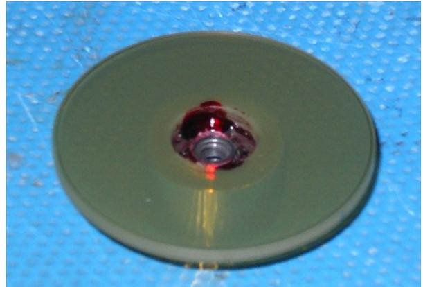
Figure 12. Rotating polarizer on its holder
