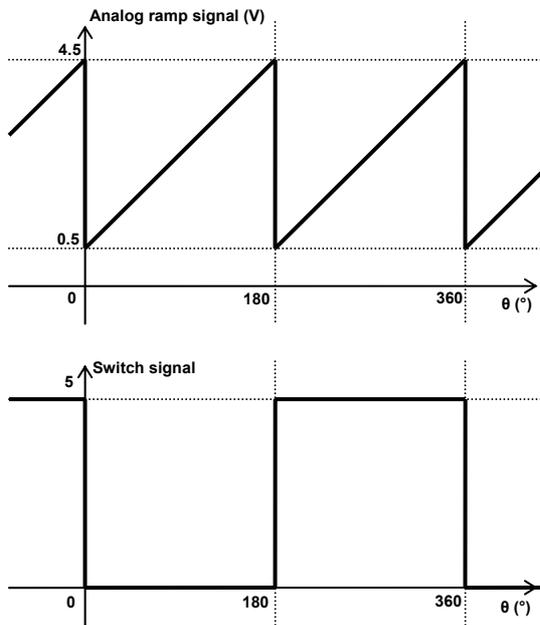
Figure 2. Output for a full analog ramp over 180° associated with a switch signal
