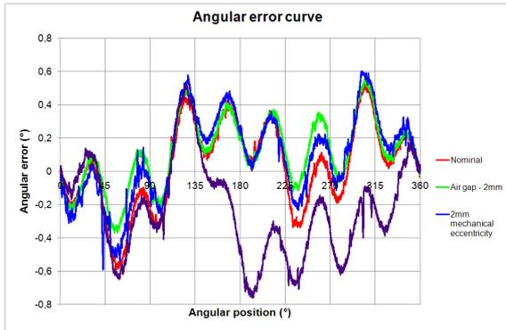
Figure 9. Geometrical defects effect on encoder's accuracy
