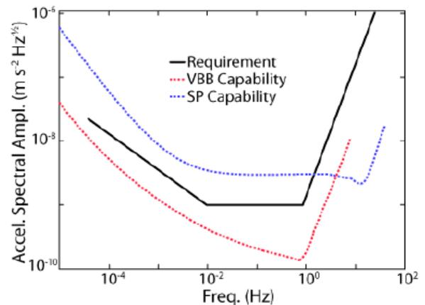
Figure 10 – GEMS-2 Seismometer's noise performance requirement and projections
