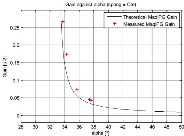
*Figure 16 – Theoretical and measured variation of the mechanical gain versus inclination of COG*
