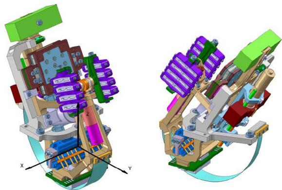
*Figure 19 – Selene-2 / GEMS-2 VBB preliminary design, including the Moon counter weight at the top of the pendulum (green part)*
