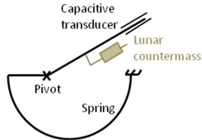
*Figure 18 – Counter mass Principle Schematic*
