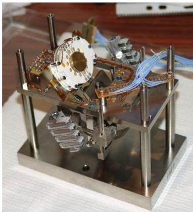
*Figure 13 – Thermal compensation device tested on VBB Mock-Up #2*
