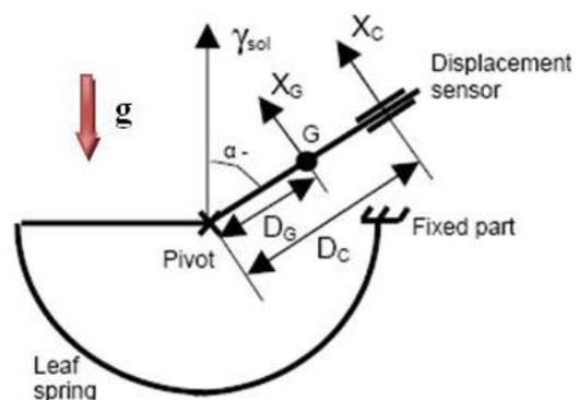
*Figure 15 – Inverted Pendulum Principle Schematic*
