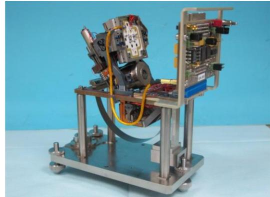
*Figure 14 – The old (Top left) and new (Top right) DCS' ceramic electrodes, and one of the two enhanced VBBs' EM integrating the new DCS (bottom)*
