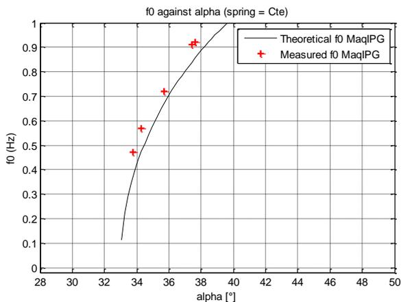
*Figure 17 – Theoretical and measured variation of the pendulum's natural oscillating frequency versus inclination of COG*
