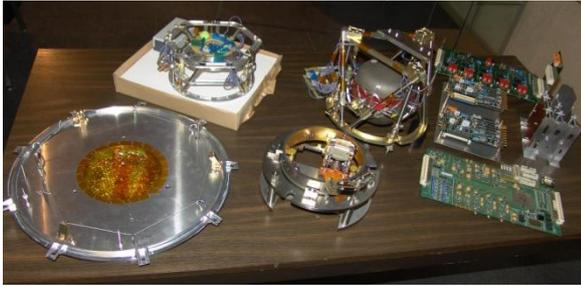
Figure 8 – ExoMars SEISmometer's Subsystems breadboards: From left to right, lander I/F with launch lock, leveling system, VBB sensor head, VBB sphere integrated in its leveling/deployment system, E-cards of the electronics, E-Box of the electronics
