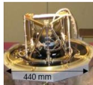
Figure 7 – ExoMars SEISmometer's Integrated Breadboard: The VBBs' Sphere (Black) mounted inside its deployment and leveling system
