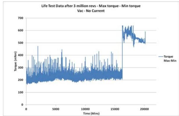
Figure 8: Torque increase at 3.2 million revs
