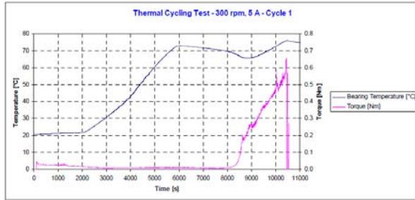
Figure 2: Torque increase above 50 deg C during testing at RUAG
