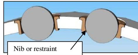
Figure 3: Schematic diagram showing design of cage inserts
