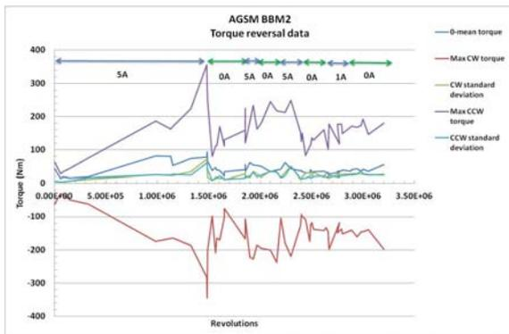
Figure 7: Summary of torques measured during reversals
