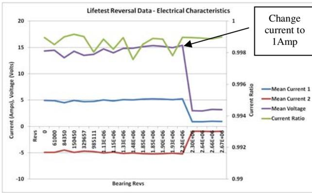
Figure 6: Summary of electrical data from torque reversals
