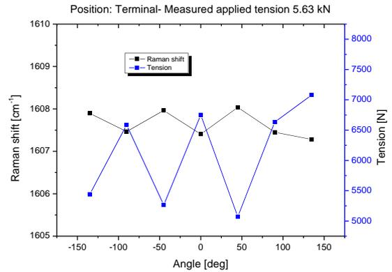
Figure 16, Preliminary Raman results on 7 positions in circumference close to the endfitting, total pretension is 6.12 kN.
