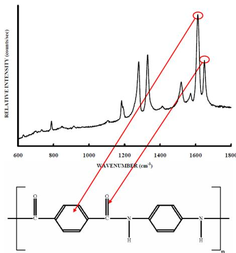
Figure 14, Raman spectrum of the non-tensioned Kevlar cable.
