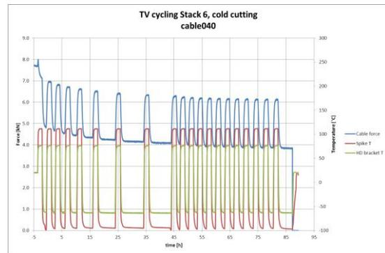
Figure 8, Thermal cycling test (20 cycles) on a 3-panel stack finalized by cutting in cold conditions.
