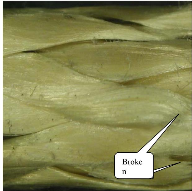
Figure 6, Photograph of the cable after test and removal of the barrel.
