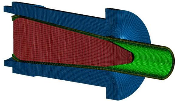
Figure 12, Model of barrel, Kevlar cable and spike
