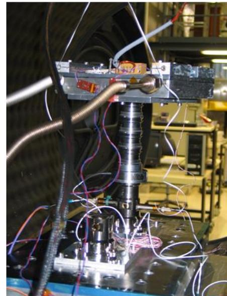
Figure 9, Set-up for 6-panel stack for hot- and cold soak in vacuum
