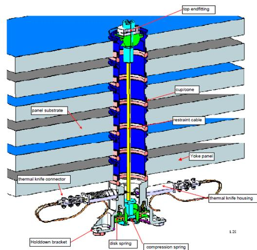
Figure 1, Cross section of a 6-panel Holddown and Release Mechanism
