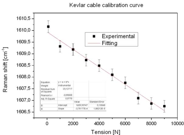
Figure 15, Characteristic curve of the tensile behaviour of the Kevlar cable (Raman peaks position difference v.s. applied tension)
