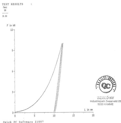
Figure 3, Proofload curve (10 kN) on cable with 110 mm length (3-panel size).
