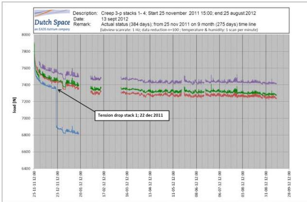
Figure 4, Relaxation test on 4 stacks at ambient conditions
