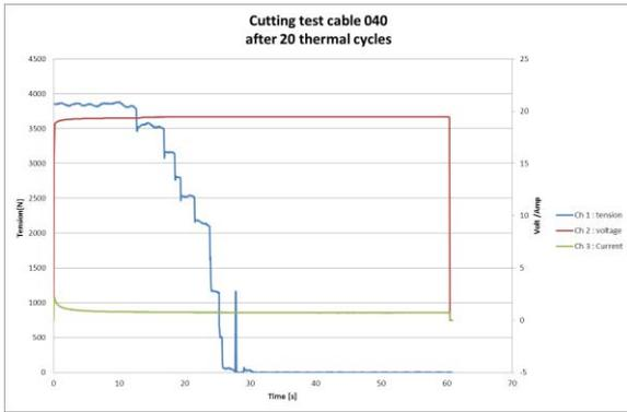
Figure 10, cutting test in cold condition after 20 thermal cycles
