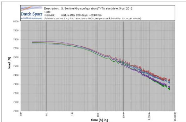
Figure 11, Relaxation test, qualification of 6-panel cable on 4 stacks
