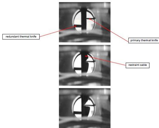
Figure 2, Thermal Knife, degrading a Kevlar Holddown cable
