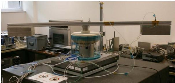
Figure 13 Microvibration test on kistler table at Astrium
