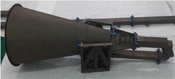
Figure 10 MGA Horn Antenna and waveguides
