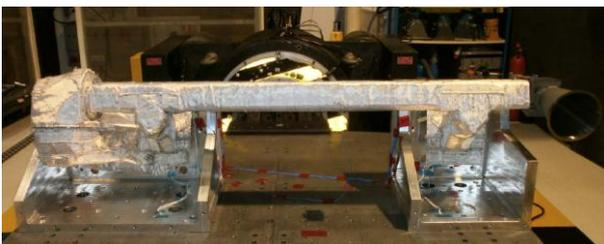
Figure 11 MGAMA STM Model in vibration test
