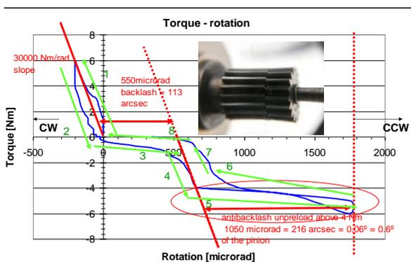
Figure 4 Torque angle behaviour of an actuator
