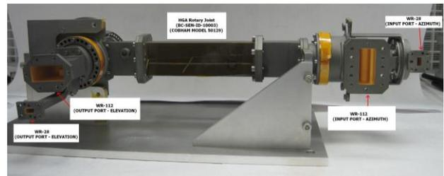
Figure 9 Rotary Joint
