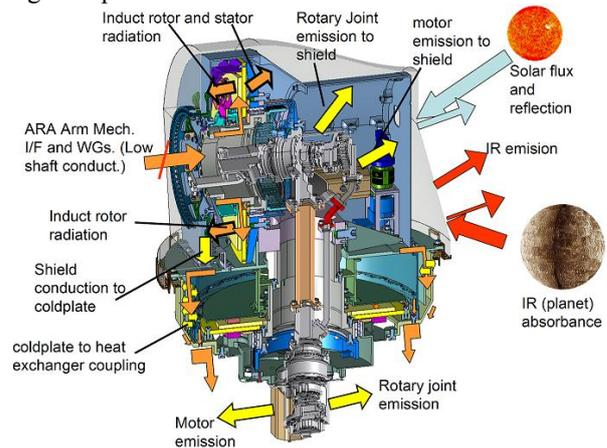
Figure 2 Thermal system schematics
