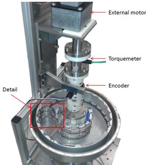
Figure 6 TWC test assembly
