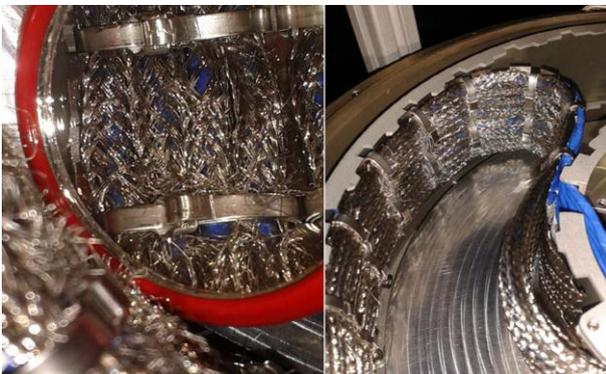
Figure 8 Problems of the first TWC during gearhead motor lifetest
