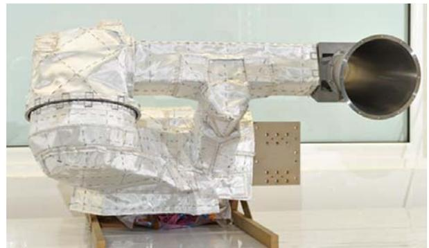
Figure 12 MGAMA Thermal model with short boom
