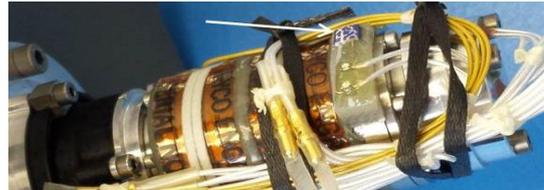
Figure 12. Motor PRT on G-10 stand-off
