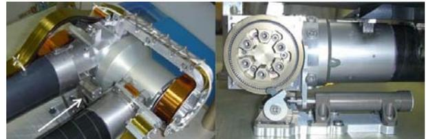
Figure 7. Elbow (left) and wrist (right) restraints
