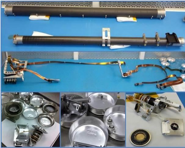
Figure 11. InSight IDA disassembled components
