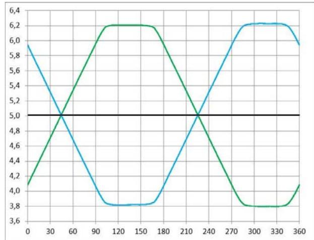
Figure 6. The  $V_{h1}$  (green) and  $V_{h2}$  (blue) signals of Fig. 4, for probes belonging to the same pair (vertical scale in Volts).
