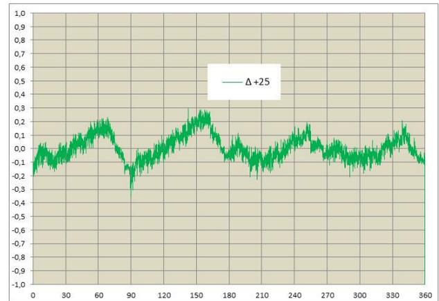
Figure 10. Total absolute error (in degrees) over the full 0-360° revolution, at 25°C.
