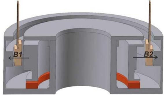
Figure 3 – The variable rotary airgap.
