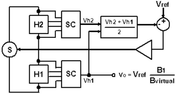
Figure 4. The feedback loop computing  $B_1/(B_1+B_2)$ .
