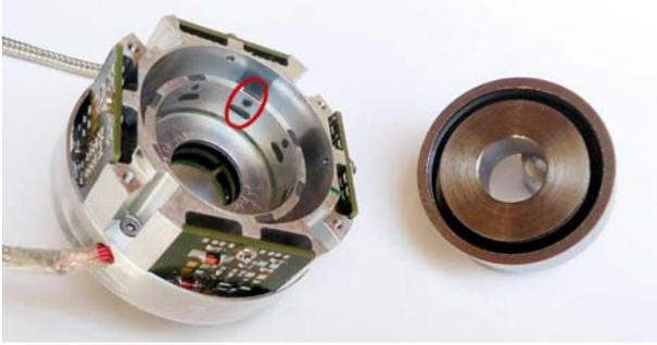
Figure 1. The Rotor separated from the Stator
