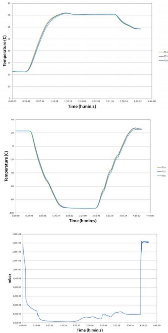
Figure 3. Time evolution of thermal-vacuum inputs: actuation at 70 °C (upper); actuation at -90°C (middle); vacuum levels (lower).
