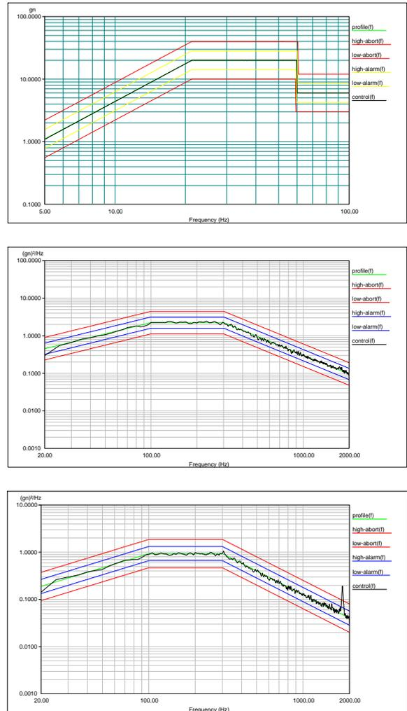
Figure 5. Time evolution of vibration inputs: sine (upper); axial random (middle); radial random (lower).
