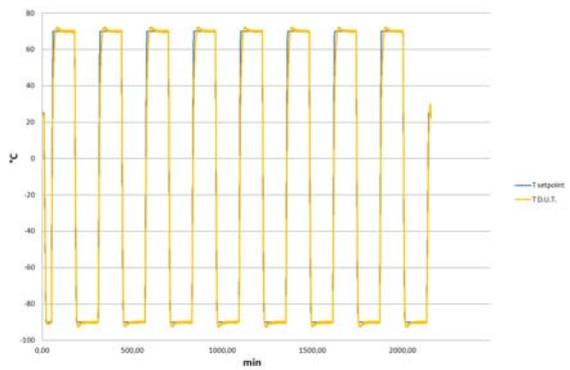
Figure 4. Time evolution of test inputs: thermal-vacuum actuation at 70 °C (left); sine vibration (right).
