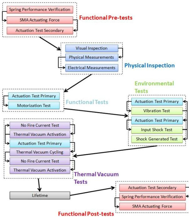
Figure 7. A proposal of qualification test campaign for REACT device.
