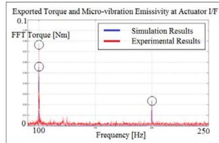
Figure 10. SMeSim Verification – Exported Torques.
