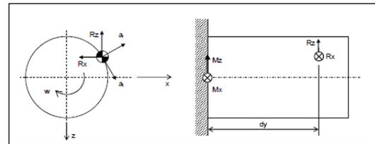
Figure 7. Example of Solar Array eccentricity model.
