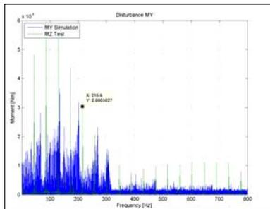
Figure 13. Output speed 1 rev/day, 64  $\mu$ steps 190 mA (The rotation axis is Y for SMeSim, Z for the test).
