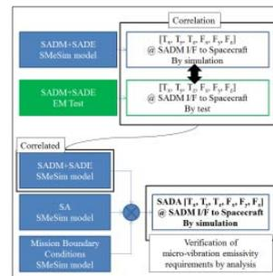
Figure 12. SMeSim Validation – Concept.
