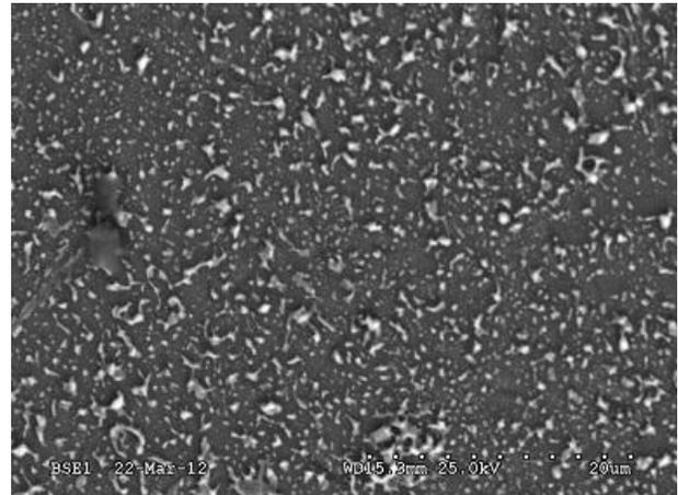
Figure 6. SEM image of 0.08 $\mu\text{m}$  indium thin-film on 52100 steel ball.
