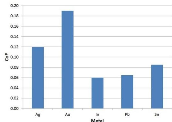
Figure 1. Friction coefficients of soft metal films in vacuum at room temperature (pin Si<sub>3</sub>N<sub>4</sub>, disc 440C, load 10N, speed 24mm/s) [3].
