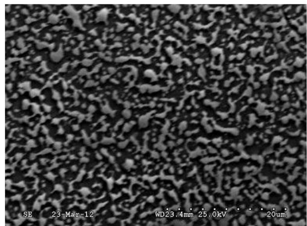
Figure 7. SEM image of 0.11 $\mu\text{m}$  indium thin-film on 52100 steel ball. Coating was produced without biasing the substrate.
