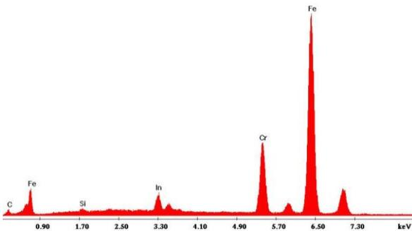
Figure 10. EDAX spectrum of running track on SOT plate, with clear indium signal. No indium peak was observed in a 'control' scan outside the running track.
