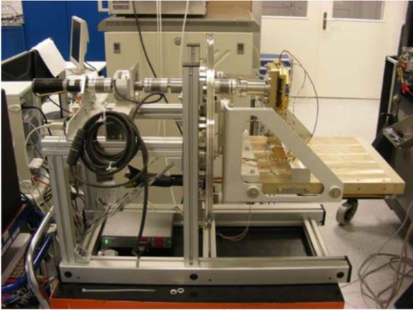
Figure 6. Potentiometer Test Set-up.
