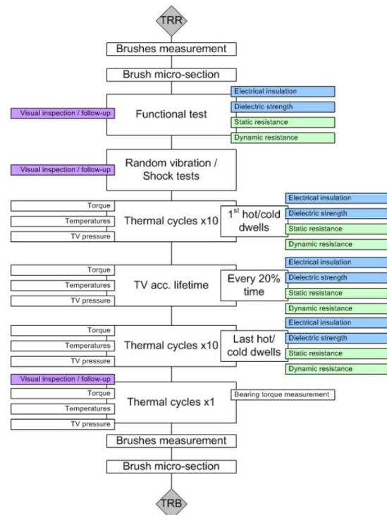
Figure 5. Slipring BB Test Sequence .
