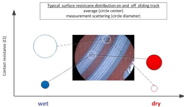
*Figure 16. Multi Point Position Sensor Surface Resistance Test Result Dry and Lubricated Sensors
