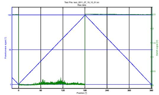
Figure 7. Position sensor Signal after 160000rev
