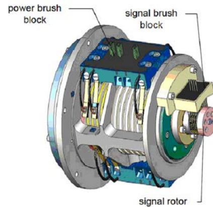
Figure 4. Slip Ring Breadboard.
