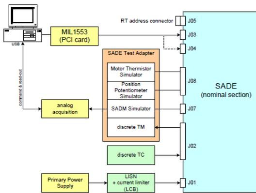
Figure 16. SADE-BB Test Setup
