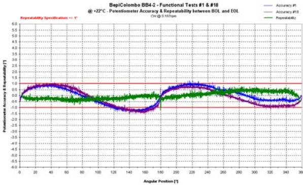
Figure 10. Deviation from Linearity BOL/EOL
