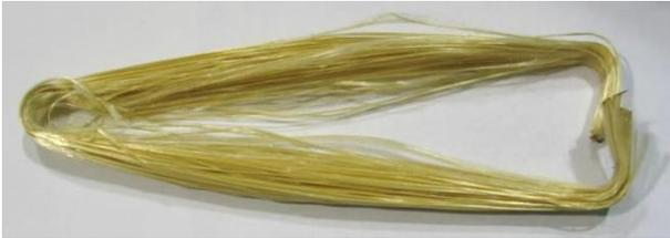
Figure 3. Looped Cord (after hotsoak and cutting test)
