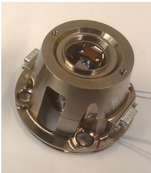
Figure 10. NELS integrated EM hardware. Bracket with Thermal Knife assembly and connectors.
