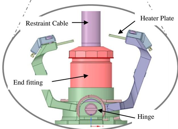
Figure 9. View on Thermal Knife assembly inside Bracket
