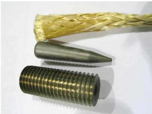
Figure 4. Spike End Fitting (after test)
